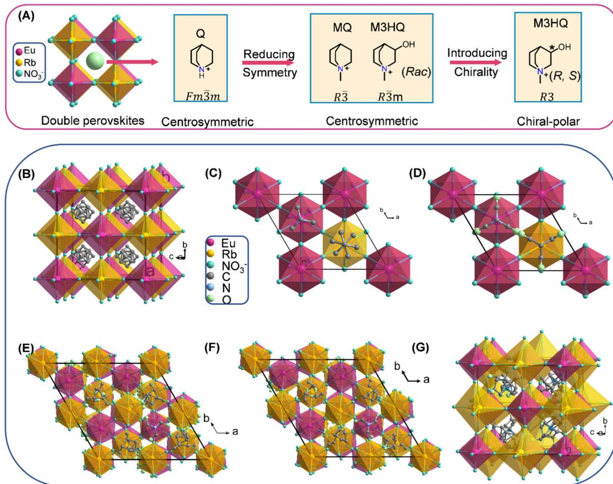
Fig. 1 Design strategy and crystal structures of 3D HREDPs. (A) Design strategy for R1 and S1. (B) (Q)<sub>2</sub>RbEu(NO<sub>3</sub>)<sub>6</sub> at 293 K. (C) (MeQ)<sub>2</sub>RbEu(NO<sub>3</sub>)<sub>6</sub> at 293 K. (D) *Rac* at 293 K. (E) S1 at 253 K. (F) R1 at 253 K. (G) R1 at 303 K. The NO<sub>3</sub><sup>-</sup> ions are simplified as balls for clarity.
