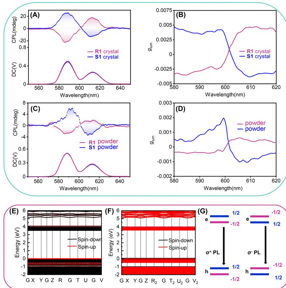
**Fig. 5** CPL properties measured at room temperature and DFT results of CPL in HREDPS. (A) CPL spectra of S1 (blue line) and R1 (red line) crystal samples excited by 397 nm. (B) The  $g_{lum}$  vs. wavelength curves of crystal samples. (C) CPL spectra of S1 (blue line) and R1 (red line) powder samples excited by 397 nm. (D) The  $g_{lum}$  vs. wavelength curves of powder samples. The DFT-calculated band structure of (E) R1 and (F) S1. (G) The mechanism of CPL.
