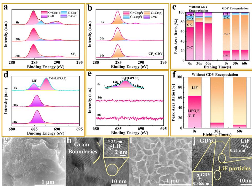
Fig. 4 C XPS spectra (a and b), F spectra (d and e) and the relative contents (c and f) stemming from the different depths given in Fig. (a and b) and (d and e) of  $\text{CF}_x$  and  $\text{CF}_x/\text{GDY}$  hybrids at the discharge state of 1.5 V, respectively. The SEM images (g and i) and HRTEM images (h and j) of  $\text{CF}_x$  and  $\text{CF}_x/\text{GDY}$  hybrids, respectively.
