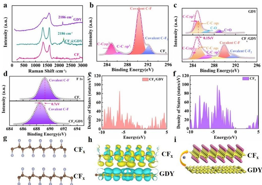
Fig. 2 Raman spectra (a) from pristine  $\text{CF}_x$ , GDY and  $\text{CF}_x/\text{GDY}$ . C 1s and F 1s spectra of  $\text{CF}_x$  (b and d), GDY (c) and  $\text{CF}_x/\text{GDY}$  (c and d). Total densities of states of  $\text{CF}_x$  (e) and  $\text{CF}_x/\text{GDY}$  (f) and the corresponding electron density differences (g and h), respectively, and the corresponding schematic diagram (i).
