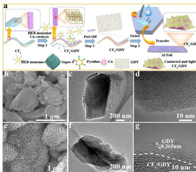
Fig. 1 (a) Schematic illustration of the synthesis of CF<sub>x</sub>/GDY. High-resolution SEM images of CF<sub>x</sub> (b) and CF<sub>x</sub>/GDY (e). TEM images (c and f) and HRTEM images (d and g) of CF<sub>x</sub> and CF<sub>x</sub>/GDY, respectively.
