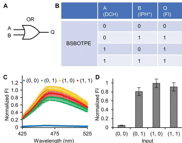
**Fig. 4** OR logic operation. (A) Symbol of logic gate. (B) Truth table. (C) The normalized fluorescence spectra of logic operation with different inputs. (D) Normalized FI at 471 nm. The concentrations of DCH (or IPH\*) and BSBOTPE used are 6  $\mu\text{M}$  and 141  $\mu\text{M}$ , respectively. Excitation wavelength was set at 350 nm.  $n = 3$ .
