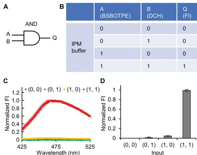
**Fig. 3** AND logic operation. (A) Symbol of logic gate. (B) Truth table. (C) The normalized fluorescence spectra of logic operation with different inputs. (D) Normalized FI at 471 nm. The concentrations of DCH and BSBOTPE used are 6  $\mu\text{M}$  and 141  $\mu\text{M}$ , respectively. Excitation wavelength was set at 350 nm.  $n = 3$ .
