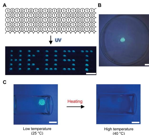
**Fig. 10** Application of molecular logic operations. (A) Storage of a 'HKUST' pattern with 'Buffer (2)' gate matrices in a 384-well plate. Top: Schematic illustration of '0' or '1' input to wells. Bottom: Fluorescent pattern 'output'. (B) Solidification of logic gates in a dextran hydrogel. (C) Application of (B) as thermo-sensors in solution. A 365-nm UV lamp was used for excitation. Scale bars, 10 mm.
