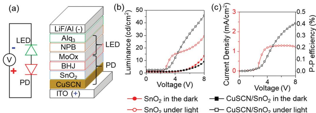
Fig. 3 Upconversion imagers with different interlayers in the photodiode stack. The incident light was at an intensity of  $5 \text{ mW cm}^{-2}$  from a 1050 nm light source. (a) Schematics of the upconversion imager with the CuSCN/SnO<sub>2</sub> bilayer. (b) Luminance of the visible light emitted from the imager *versus* the applied bias. (c) Current density and photon-to-photon upconversion efficiency *versus* the applied bias.
