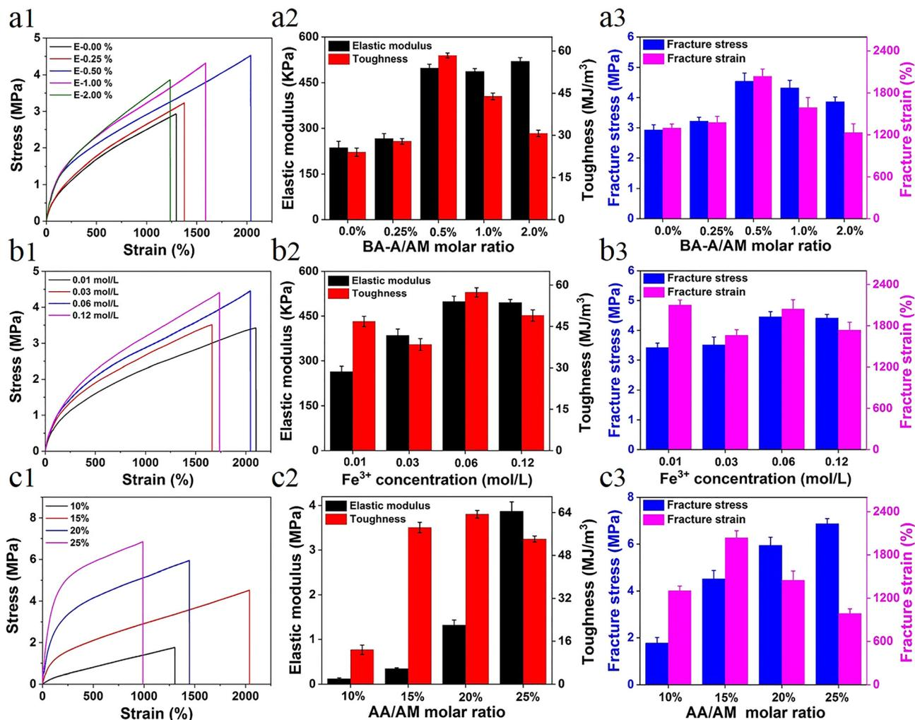
Fig. 1 Tensile curves with different contents of (a1) BA-A/AM, (b1)  $\text{Fe}^{3+}$ , and (c1) AA/AM; variation of the content of elastic modulus and toughness of (a2) BA-A/AM, (b2)  $\text{Fe}^{3+}$ , and (c2) AA/AM; and variation of the content of fracture stress and strain of (a3) BA-A/AM, (b3)  $\text{Fe}^{3+}$ , and (c3) AA/AM.
