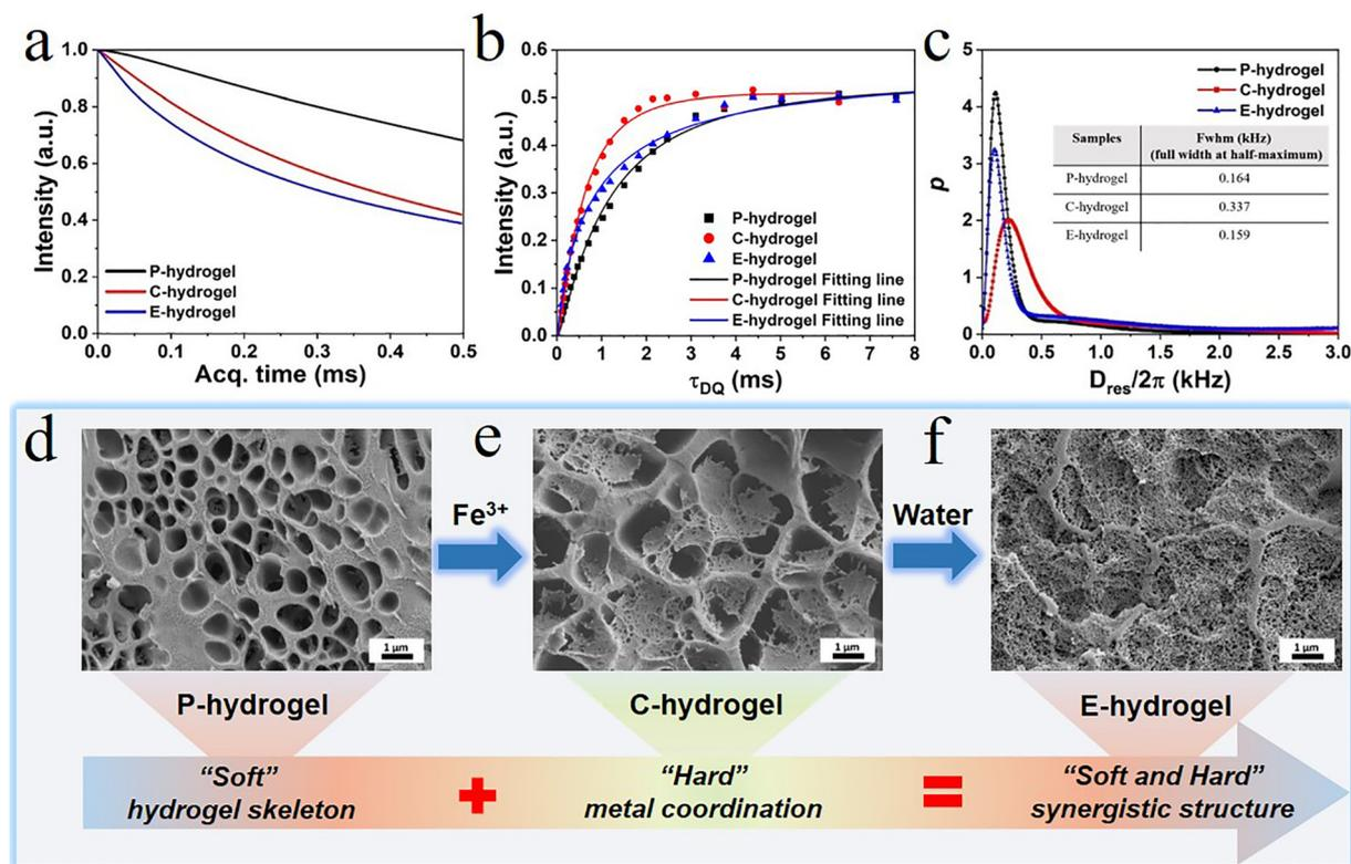
Fig. 3 (a) Low-field MSE-FID NMR signal; (b) normalized DQ intensity as a function of DQ excitation time; (c)  $D_{\text{res}}$  distribution curves as obtained from the fitting on the normalized DQ curves; and SEM images of (d) P hydrogel, (e) C-hydrogel, and (f) E-hydrogel.
