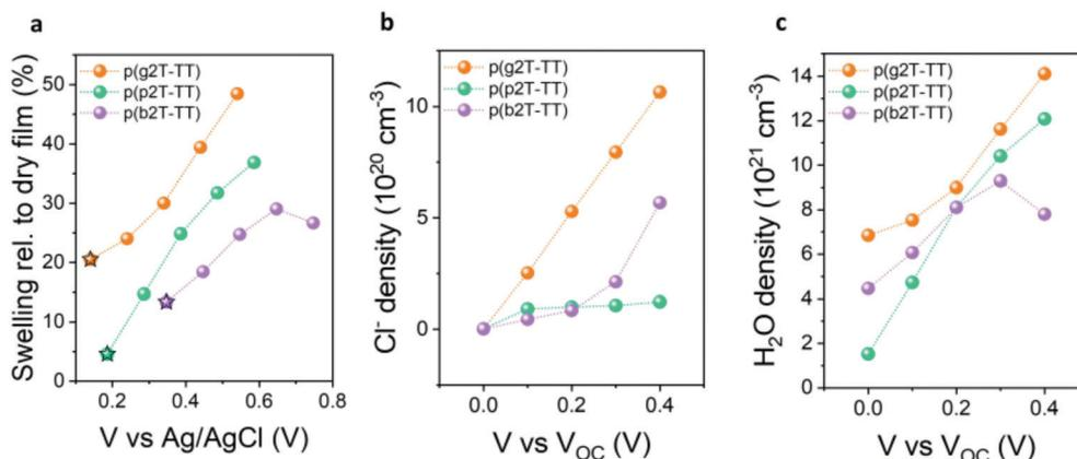
Fig. 3 (a) Polymer swelling relative to the corresponding dry state. Star symbols correspond to the swelling values of the film at  $V_{\text{OC}}$  conditions (*i.e.*, passive swelling). The voltage values are plotted vs. Ag/AgCl. (b) Chloride ion and (c) water molecule density in the conjugated polymer film following electrochemical doping at various potentials against  $V_{\text{OC}}$ .  $V_{\text{OC}}$  values are 0.14 V for p(g2T-TT), 0.19 V for p(p2T-TT), and 0.35 V for p(b2T-TT).
