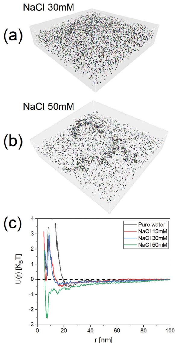
Fig. 5 The effect of NaCl on the potentials of mean force of **NP2**. (a) Tomogram of **NP2** at the NaCl 30 mM. (b) Tomogram of **NP2** at the NaCl 50 mM. (c) Comparison of the resulted potentials of mean force at various NaCl concentrations.
