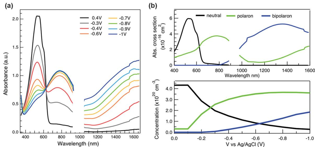
**Fig. 3** (a) *In situ* absorbance spectra of the spin-coated P3HT film at different applied voltages versus Ag/AgCl electrode in 0.1 M KPF<sub>6</sub>/water in steady state conditions. (b) Component spectra (top) and voltage-dependent concentrations (bottom) of the neutral, polaronic and bipolaronic species of electrochemically doped P3HT, as obtained from soft-modeling MCR-ALS analysis of the spectro-electrochemistry spectra.
