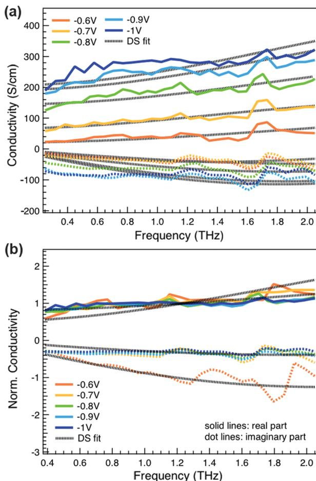
Fig. 2 (a) Complex conductivity spectra of electrochemically doped P3HT at different oxidation potentials *versus* Ag/AgCl. The real and imaginary parts are shown with solid and dotted lines. (b) Normalized real (solid) and scaled imaginary (dashed) parts of the conductivity at different applied voltages. The fit results from the Drude–Smith model are shown with black dotted lines.
