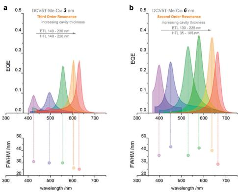
Fig. 9 EQE curves and correlated FWHM of cavity enhanced OPDs with (a) 3 nm thick photo-absorbing layer and third order resonance (m = 3) and (b) 6 nm thick photo-absorbing layer and second order resonance (m = 2). The tunable enhanced wavelengths are realized by varying the thickness of ETL and HTL. Reproduced with permission.<sup>81</sup> Copyright 2019, American Chemical Society.
