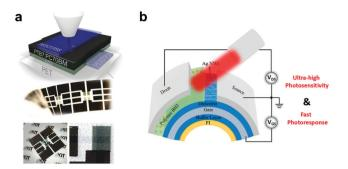
(a) Schematic structure and photographs of fully-printed ITO-free OPDs on PET foil showing their semi-transparency and mechanical flexibility.<sup>216</sup> (b) Device structure of flexible PT-OPDs with ultrashort channel length. 217 (a) Reproduced with permission.<sup>216</sup> Copyright 2015, WILEY-VCH GmbH. (b) Reproduced with permission.<sup>217</sup> Copyright 2018, American Chemical Society.
