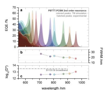
Fig. 11 Solution processed PBTTT:PC<sub>61</sub>BM CT-OPDs based on the second order resonance. (a) Simulated and experimental (hatched) resonance wavelength and correlated EQE curves. The wavelength tunability in range of 650-910 nm was realized by varying the active layer thickness from 290-440 nm. (b) Corresponding FWHM and (c) D\*. Reproduced with permission.<sup>74</sup> Copyright 2017, WILEY-VCH GmbH.
