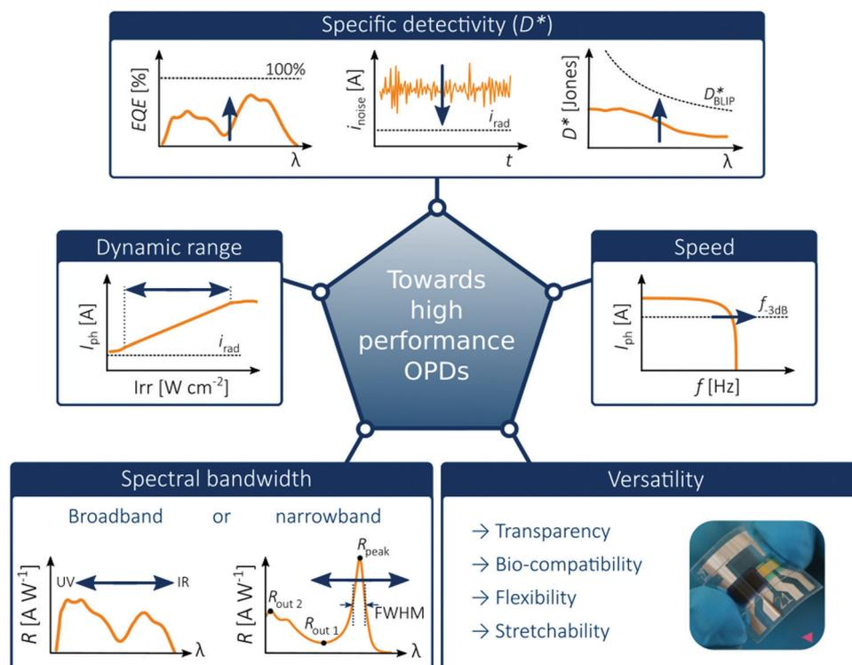
Fig. 2 Illustration of challenges for emerging OPDs. The picture of the flexible OPD is reproduced with permission,<sup>27</sup> copyright 2017, Springer Nature.
