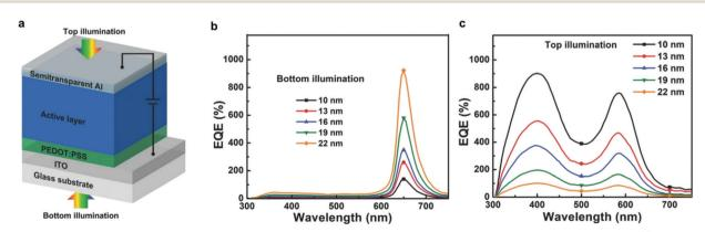
Fig. 7 (a) CIN-PM-OPD structure. EQE of the CIN-PM-OPD under (b) bottom and (c) top illumination. Reproduced with permission. 193 Copyright 2018, Wiley-VCH GmbH.
