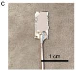
Fig. 1 (a) Optical image of a representative restacked MoS<sub>2</sub> film on a nitrocellulose membrane. (b) SEM cross sectional image of a representative restacked MoS<sub>2</sub> film. (c) Optical image of an electrode prepared by transferring a restacked MoS<sub>2</sub> film onto a gold substrate. The edges of the electrode were sealed using silver paint.
