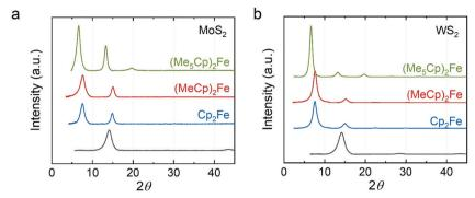
Fig. 2 XRD of metallocene intercalated (a) MoS<sub>2</sub> and (b) WS<sub>2</sub>. Green: decamethylferrocene-intercalated; red: 1,1'-dimethylferrocene-intercalated; blue: ferrocene-intercalated; dark gray: restacked.
