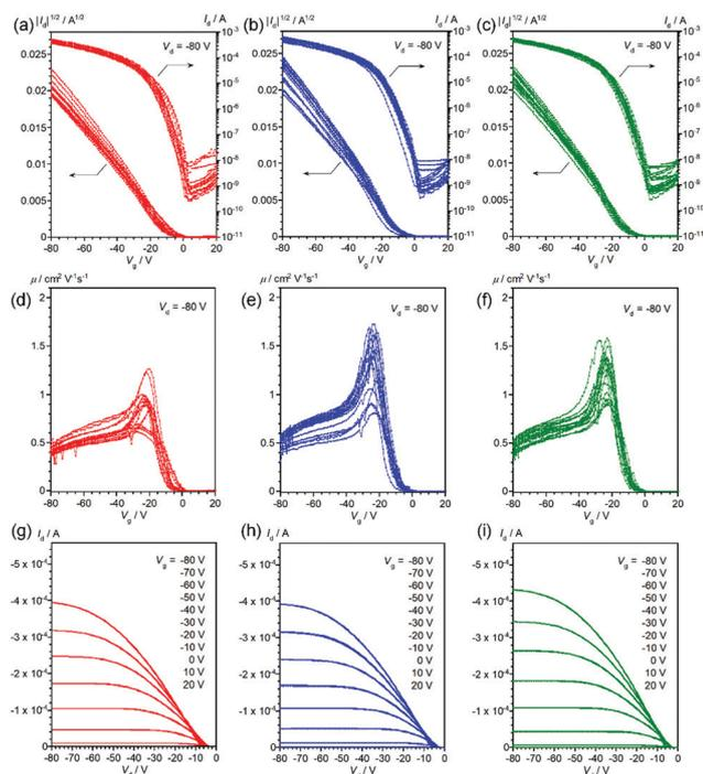
**Fig. 5** Transfer curves (a–c), gate-voltage-dependence of mobility (d–f), and output curves (g–i) of OFET devices based on spin-coated *R*- (red), *S*- (blue), and *rac*- (green) EH-DNTT thin films, respectively. Transfer and gate-voltage-dependent mobility curves are overlaid for more than twelve devices.
