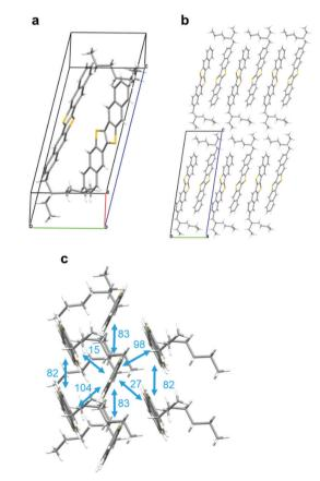
Fig. 2 Crystal structure of S-EH-DNTT. (a) Molecular structures of two crystallographically-independent molecules, (b) lamella structure, and (c) the herringbone packing structure observed in the lamella layers and the calculated intermolecular electronic coupling (transfer integrals, meV, in cvan) of the HOMO
