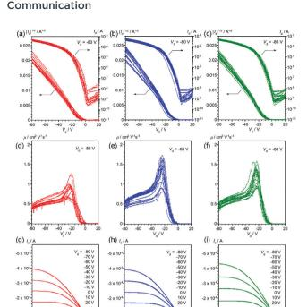
Fig. 5 Transfer curves (a-c), gate-voltage-dependence of mobility (d-f), and output curves (q-i) of OFET devices based on spin-coated R- (red), S- (blue), and rac- (green) EH-DNTT thin films, respectively. Transfer and gate-voltagedependent mobility curves are overlaid for more than twelve devices.
