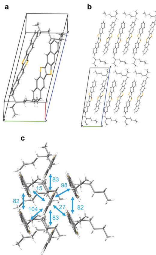
Fig. 2 Crystal structure of *S*-EH-DNTT. (a) Molecular structures of two crystallographically-independent molecules, (b) lamella structure, and (c) the herringbone packing structure observed in the lamella layers and the calculated intermolecular electronic coupling (transfer integrals, meV, in cyan) of the HOMO.
