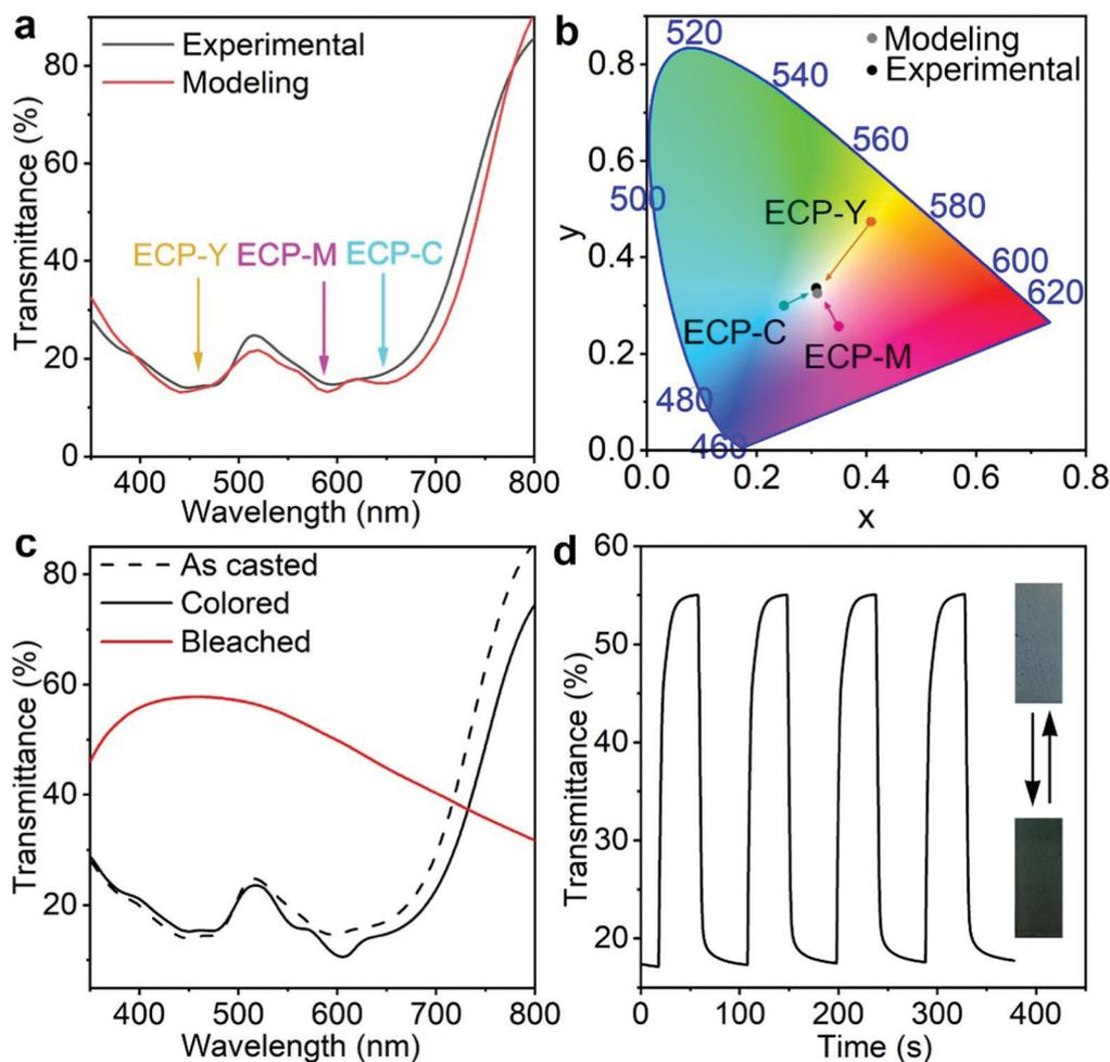
**Fig. 3** Neutral grey electrochromic polymer from a triple-layer ECP. (a) Experimental vs. modeling spectra of the triple-layer ECP. (b) Chromaticity values extracted from the modeling and experimental spectra of the triple-layer ECP. The  $xy$  values of the constituent single-layer ECP-C, ECP-M, ECP-Y are also shown alongside. (c) Spectroelectrochemistry and (d) double potential step chronoabsorptometry of the triple-layer ECP.
