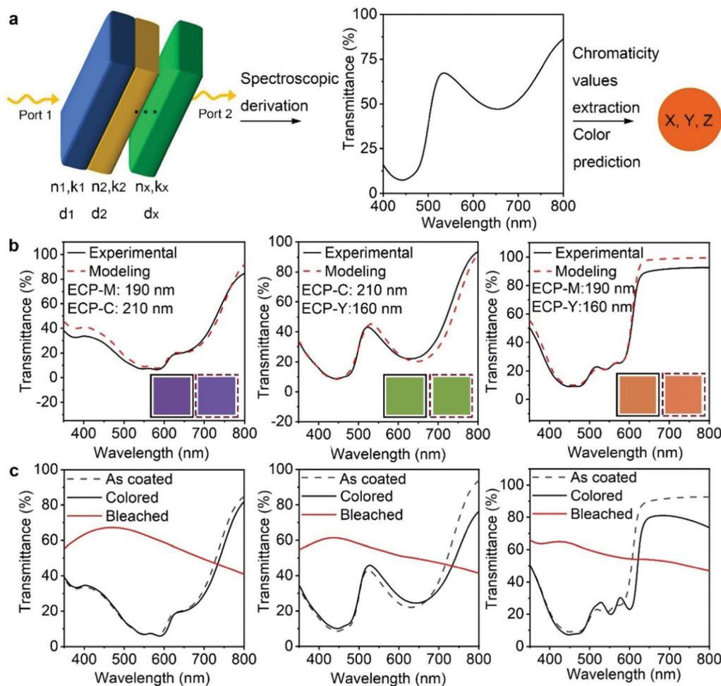
**Fig. 2** Optical modeling-guided double-layer ECP stacking. (a) Workflow of the optical modeling. (b) Experimental vs. modeling spectra of the double-layer ECPs consisting of various polymer thicknesses. The colors in the solid and dashed boxes are predicted by experimental and modeling spectra, respectively. (c) Spectroelectrochemistry of the double-layer ECPs.
