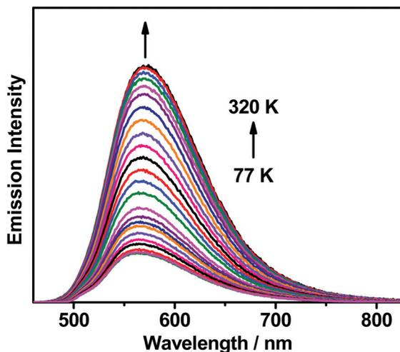
Fig. 3 Emission spectra of the thin film of 20 wt% **1** doped in MCP upon increasing the temperature from 77 to 320 K.
