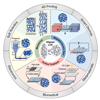
Fig. 1 Nematic-isotropic phase transition of mesogens in a liquid crystal elastomer (LCE) network gives rise responsive and reversible Various mesogen alignment strategies include mechanical alignment, magnetic/electric field alignment, and surface treatment.
