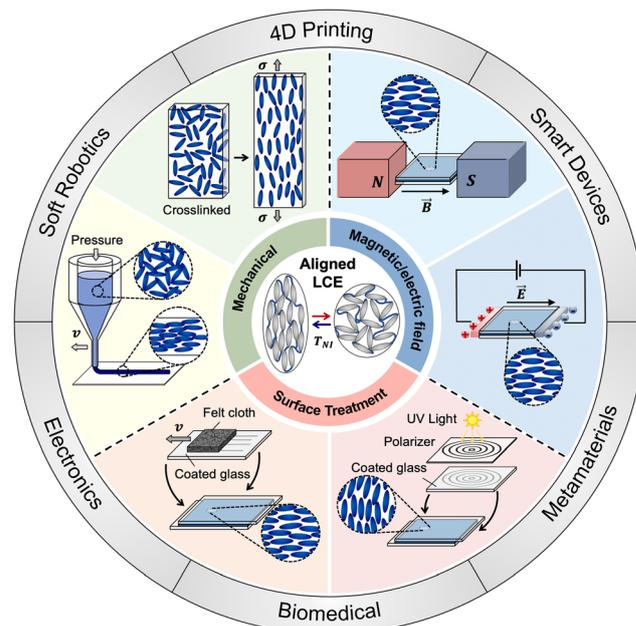
**Fig. 1** Nematic-isotropic phase transition of mesogens in a liquid crystal elastomer (LCE) network gives rise responsive and reversible deformation. Various mesogen alignment strategies include mechanical alignment, magnetic/electric field alignment, and surface treatment.
