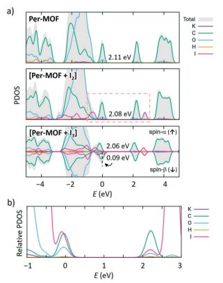
Fig. 5 a) Atom-projected density of states (PDOS) and bandgap values calculated for Per-MOF, [Per-MOF +  $I_2$ ] and [Per-MOF +  $I_3$ ] at the HSE06 level. Spin- $\alpha$  and spin- $\beta$  channels (with their corresponding bandgaps) are indicated in [Per-MOF  $+ I_3$ ]. The Fermi level was set to the valence band maximum. b) Relative PDOS of [Per-MOF + I2] calculated as the PDOS divided by the number of atoms of each type in the unit cell.
