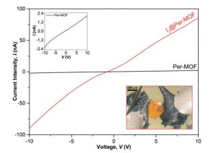
Fig. 7 Representative current (I)-voltage (V) plot for crystal devices of Per-MOF (black) and I2@Per-MOF (red) at 300 K. The inset in the upper panel shows the Per-MOF I-V curve with a proper scale. The image in the lower panel shows a micrograph of an I2@Per-MOF crystal with Ag epoxy + carbon-based paste contacts.
