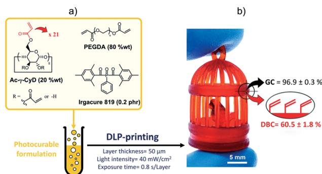
**Fig. 1** a) Photocurable Ac- $\gamma$ -CyD/PEGDA formulation studied in this work, and b) DLP-printed part (methyl red dye added to increase the printing resolution), characterized by a GC close to 97% but with a DBC below 61%.
