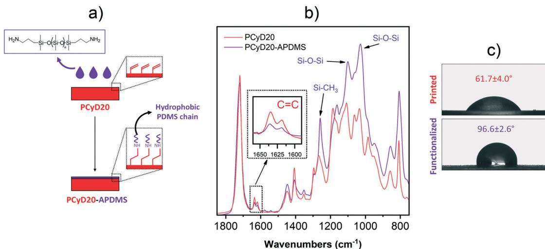
**Fig. 2** a) Schematic representation of the surface-grafting of A-PDMS onto the printed sample PCyD20 following the aza-Michael reaction pathway; b) ATR spectra of the printed and functionalized samples, PCyD20 and PCyD20-APDMS, respectively, with a detailed view of the C=C stretching vibration at  $1633\text{ cm}^{-1}$  before and after the surface modification and c) water contact angles on the surface of both the printed and functionalized samples.
