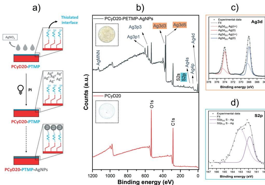
**Fig. 6** a) Schematic representation of the photoreduction of Ag ions and the immobilization of AgNPs onto the free pendent –SH groups on the thiolated PCyD20-PETMP interface via S–Ag bridging-bonds; b) survey XPS spectra of the printed sample before (PCyD20) and after the photografting of AgNPs (PCyD20-PETMP-AgNPs), with inset photographs of the samples; and high resolution S2p (c) and Ag3d (d) spectra showing the experimental data, the best fitting analysis, and the deconvolution.
