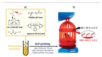
Fig. 1 a) Photocurable Ac-γ-CyD/PEGDA formulation studied in this work, and b) DLP-printed part (methyl red dye added to increase the printing resolution), characterized by a GC close to 97% but with a DBC below 61%
