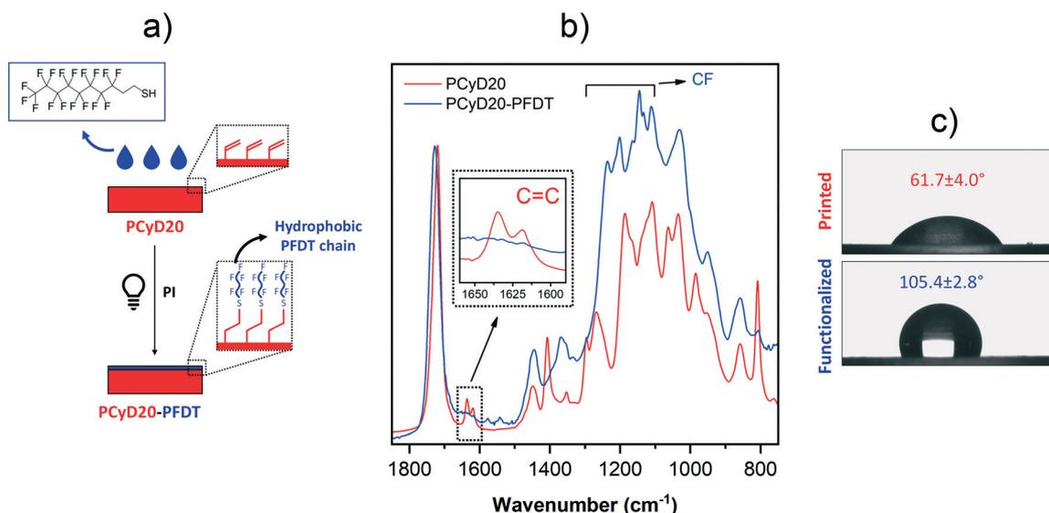
**Fig. 3** a) Schematic representation of the surface-grafting of PFDT onto the printed sample PCyD20 following the thiol-ene addition pathway; b) ATR spectra of the printed and functionalized samples, PCyD20 and PCyD20-PFDT, respectively, with a detailed view of the C=C stretching vibration at  $1633\text{ cm}^{-1}$  before and after the surface modification and c) water contact angles on the surface of both the printed and functionalized samples.
