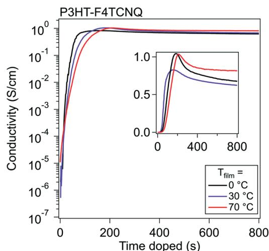
**Fig. 2** *In situ* conductivity curves of F4TCNQ-doped P3HT. The  $\sigma$  for P3HT over the course of doping with F4TCNQ is shown for three different  $T_{\text{film}}$ . The semilog plot shows that  $\sigma$  rises five orders of magnitude in around two minutes, and the linear inset details the form of the drop in  $\sigma$  past  $\sigma_{\text{max}}$ .
