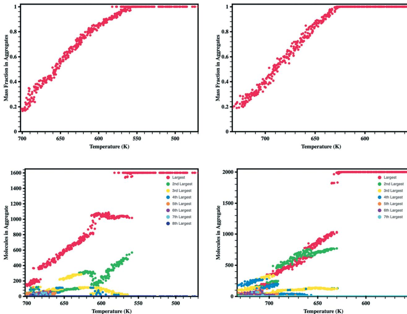
Fig. 4 (Top) Fraction of total simulation mass present within aggregates versus free molecules for *antiADT* (left) and *synADT* (right). (Bottom) Total number of molecules within the largest aggregates present within the simulation boxes prior to aggregates coalescing. Note differing X-axis scales for *antiADT* and *synADT* due to aggregate formation initiating at different temperatures (Fig. 1).
