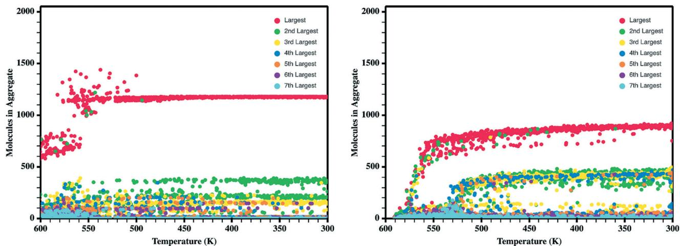
Fig. 5 Number of molecules in each crystalline aggregate in *antiADT* (left) and *synADT* (right) as the simulation boxes are cooled. Note a total of 1600 *antiADT* molecules and 2000 *synADT* molecules.
