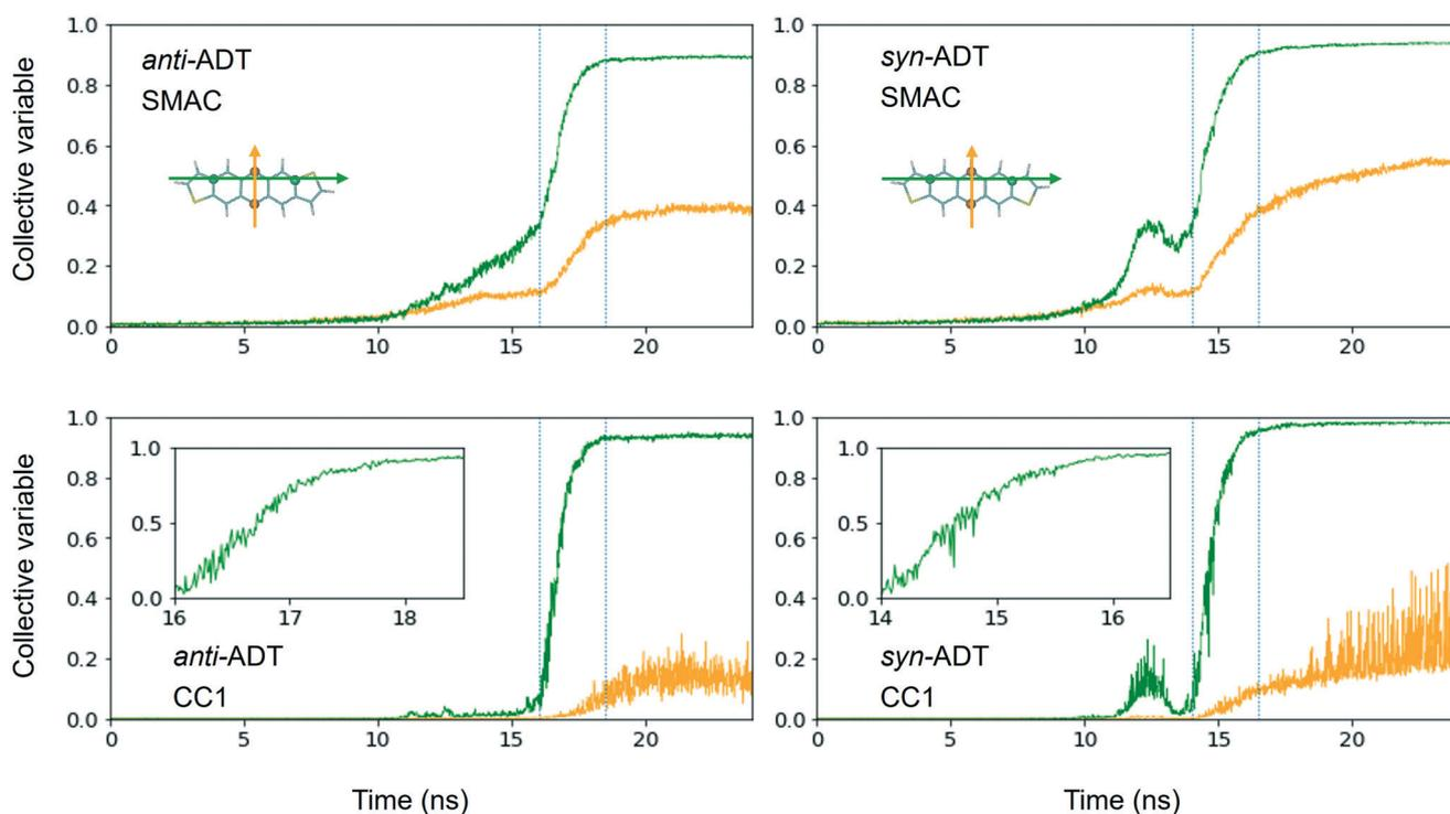
**Fig. 6** Normalized crystallinity descriptor collective variables (CV) SMAC (top row) and CC1 (bottom row) derived for the cooling of *anti*ADT and *syn*ADT as a function of simulation time in terms of the long-axis (green) and short-axis (yellow) vectors. The inserts in the figures in the bottom row highlight the CV changes during crystallization, which fall between the dotted lines in the full images.
