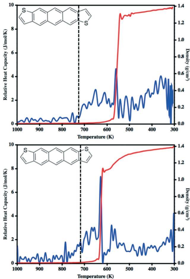
Fig. 3 Relative heat capacity (blue) and simulation box density (red) of *anti*ADT (top) and *syn*ADT (bottom) as the system is cooled from 1000 K to 300 K. The experimental melting points of the *anti*ADT (725 K) and *syn*ADT (720 K) are highlighted with dashed, black lines.
