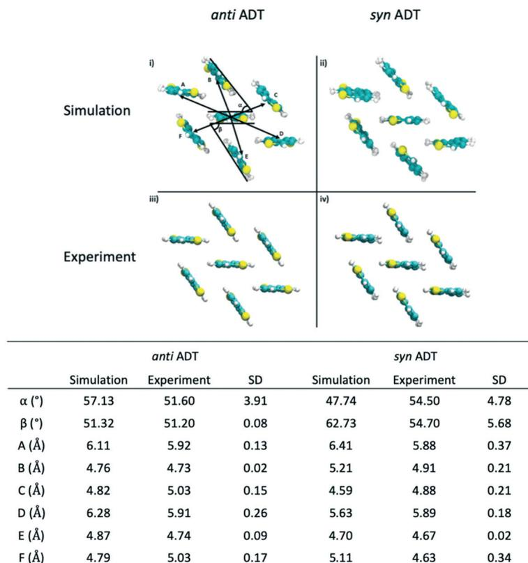
**Fig. 8** Comparison of crystalline packing of *anti*ADT and *syn*ADT as extracted from a series of snapshots after simulation box crystallization to the experimentally reported crystal structure. Molecular distances and angles are reported in table with standard deviations for each angle and distance.
