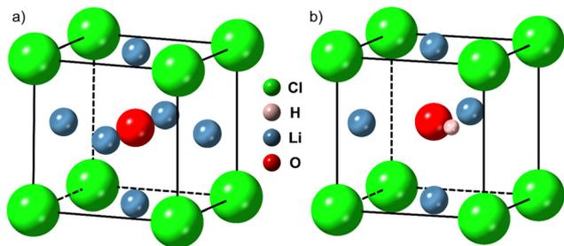
Fig. 1 Crystallographic structures of (a)  $\text{Li}_3\text{OCl}$  ( $Pm\bar{3}m$ ) and (b)  $\text{Li}_2\text{OHCl}$  ( $Pmc2_1$  below  $\sim 32^\circ\text{C}$ ,  $Pm\bar{3}m$  above).<sup>7,16–18</sup> Generated using CrystalMaker<sup>®</sup>: CrystalMaker Software Ltd, Oxford, England ([www.crystallmaker.com](http://www.crystallmaker.com)).
