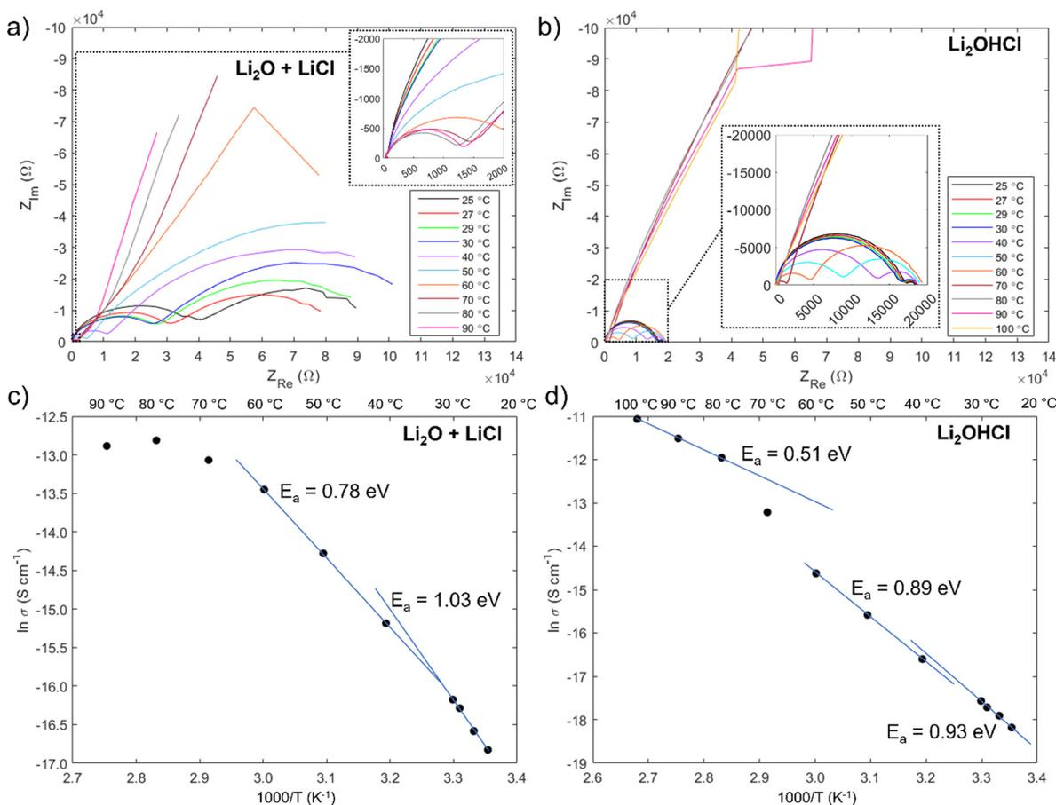
Fig. 7 Results of through-plane impedance measurements performed at temperatures between  $25\text{ }^\circ\text{C}$  and  $90/100\text{ }^\circ\text{C}$ . Nyquist plots for the films deposited from  $\text{Li}_2\text{O} + \text{LiCl}$  and  $\text{Li}_2\text{OHCl}$  targets are shown in (a) and (b) respectively; (c) and (d) show the corresponding Arrhenius plots and activation energies calculated from the linear fit lines.
