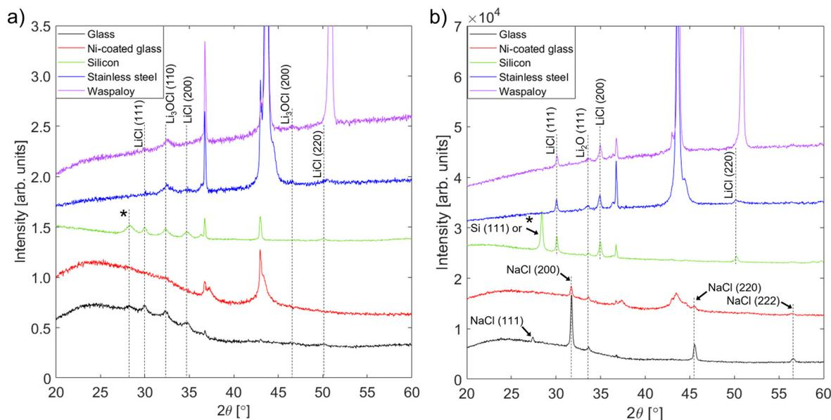
Fig. 2 XRD patterns of films deposited from Li<sub>2</sub>O + LiCl targets onto several different substrate materials: (a) in the as-deposited condition and (b) after annealing at 250 °C for 1 hour. Peaks marked \* correspond to impurity phases from the precursor mixture such as KCl. Unlabelled peaks are from the substrate or sample holder; the differing intensities of holder peaks are due to differences in the lateral positioning of samples within the holder.
