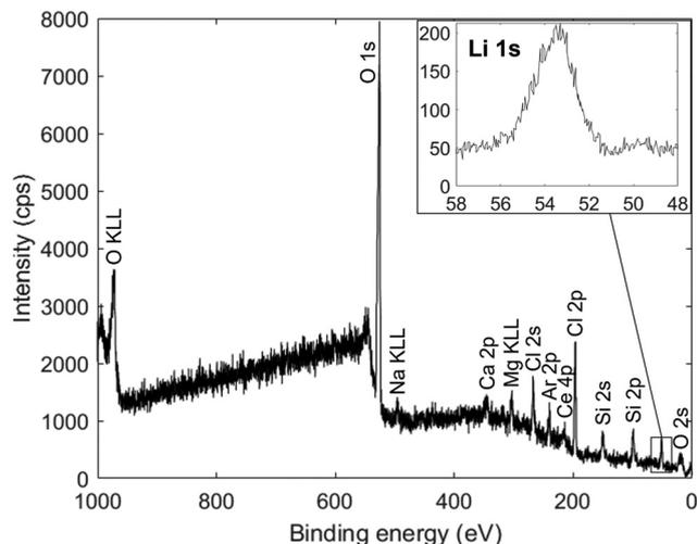
**Fig. 5** XPS spectrum of a film deposited from an  $\text{Li}_2\text{O} + \text{LiCl}$  target onto a glass substrate, measured after etching the film surface using a 4 kV Ar-ion beam for 40 minutes to remove surface impurities and carbon-rich layers. The inset shows a high resolution plot of the Li 1s peak. Unlabelled peaks do not correspond to any probable film impurities and are thus attributed to contamination from the XPS chamber.
