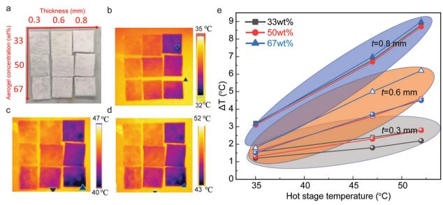
Fig. 3 (a) Optical images of the samples on the hotplate. The scale bar is 10 mm. (b-d) Infrared images of various samples at heating temperatures of 35 °C, 47 °C, and 52 °C. (e) Temperature difference between various composite membranes and the stage vs. hot stage temperature.
