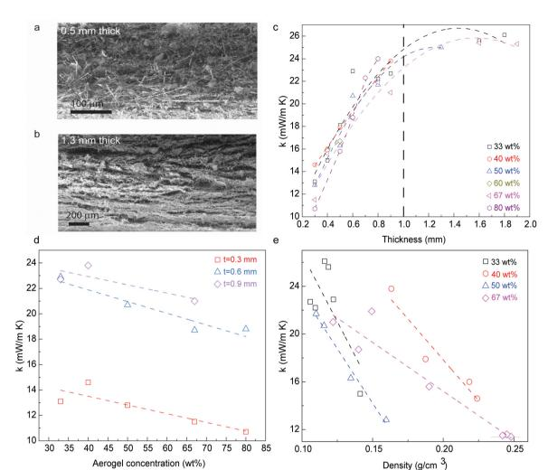
Fig. 2 (a) Cross-sectional SEM image of the membrane with a thickness of 500 µm. (b) Cross-sectional SEM image of the membrane with a thickness of 1.3 mm. (c) Thermal conductivity vs. thickness of the membrane with different concentrations. (d) Thermal conductivity vs. aerogel concentration for membranes with thicknesses of 0.3 mm, 0.6 mm and 0.9 mm. (e) Thermal conductivity vs. density for membranes with different aerogel concentrations.
