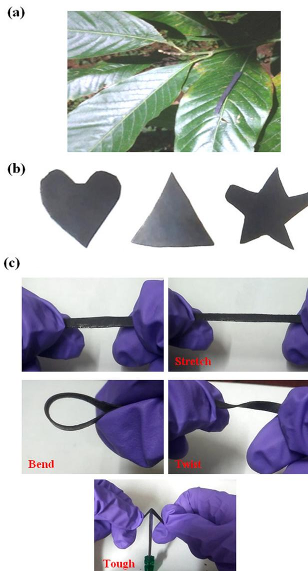
**Fig. 2** The robustness and resilience of the graphite nanoflake/nitrile elastomer nanocomposite strain sensors. (a) Graphite nanoflake/nitrile elastomer nanocomposite sensor placed on a leaf to demonstrate its lightweight features. (b) Different shapes of the graphite nanoflake/nitrile elastomer nanocomposites. (c) Stretching, bending, twisting, and toughness of the graphite nanoflake/nitrile elastomer nanocomposite strain sensors.
