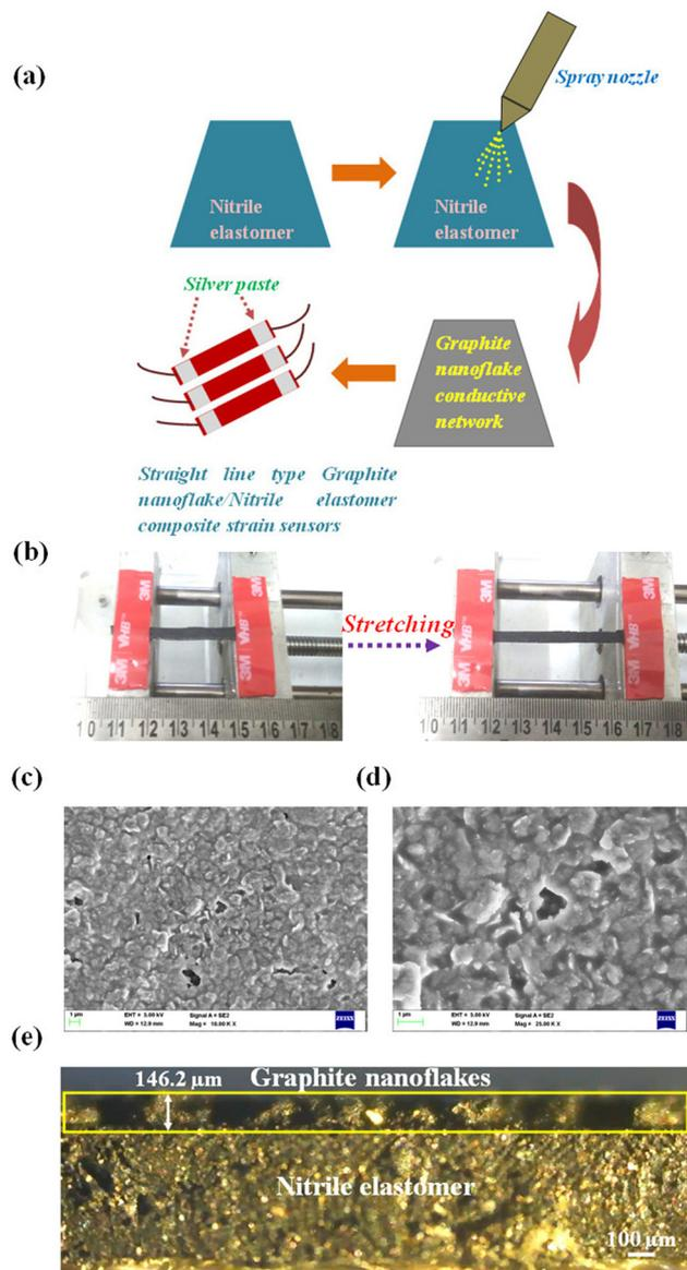
**Fig. 1** (a) Scheme of the construction process of the ultrasensitive graphite nanoflake/nitrile elastomer nanocomposite strain sensors. (b) The graphite nanoflake/nitrile elastomer nanocomposite strain sensor demonstrated high stretchability during the application of tensile strains. (c) The SEM image of the graphite nanoflake conductive network. (d) A zoomed-in SEM image of (c). (e) Cross-sectional optical image of graphite nanoflake/nitrile elastomer nanocomposite strain sensors.
