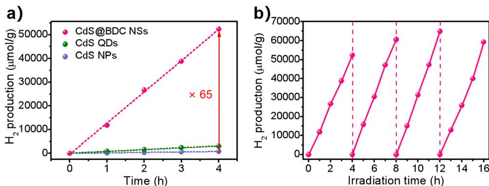
**Fig. 4** (a) Comparison of the photocatalytic H<sub>2</sub>-evolution activities of CdS@BDC NSs, CdS QDs and CdS NPs. (b) Cycling stability for the CdS@BDC NS photocatalysts.
