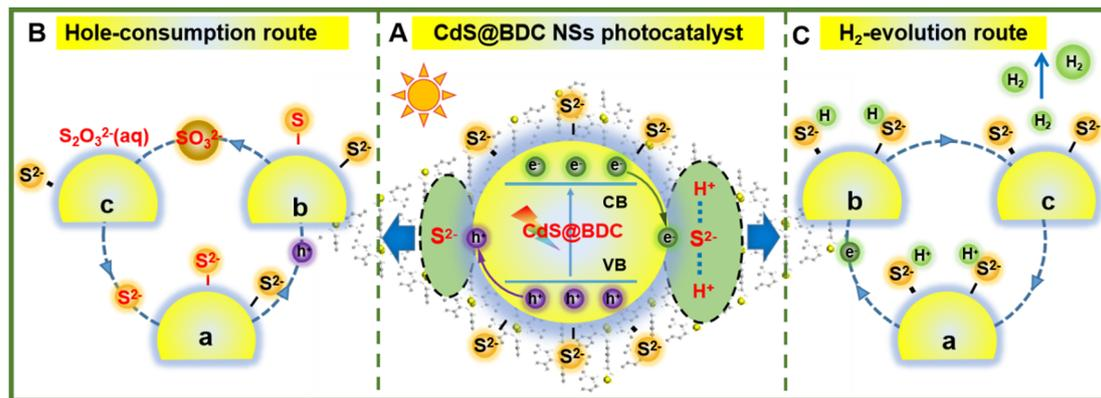
Fig. 6 Schematic illustration of the  $S^{2-}$ -mediated mechanism in CdS@BDC NSs: (A)  $S^{2-}$ -mediated interfacial charge transfer and separation in the CdS@BDC NSs, (B) hole-consumption route by  $S^{2-}/SO_3^{2-}$  ions, and (C)  $H_2$ -evolution reaction route on the adsorbed  $S^{2-}$  ions as the catalytic active sites.
