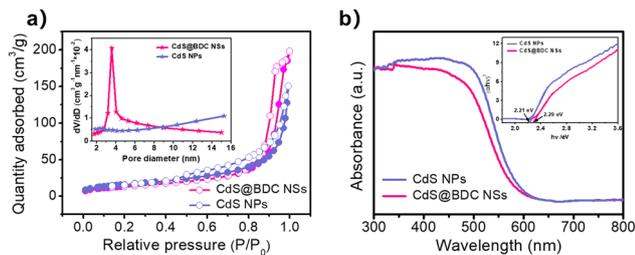
**Fig. 3** (a) Nitrogen adsorption/desorption isotherms of the CdS@BDC NSs and CdS NPs (the inset exhibits corresponding pore size distribution curves). (b) UV-vis diffuse absorption spectra and their calculated band gap (inset) of the CdS@BDC NSs and CdS NPs.
