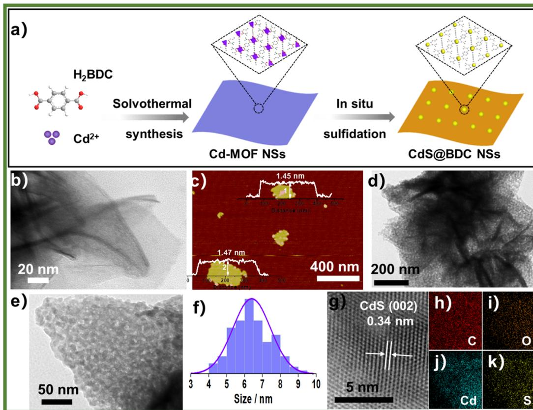
**Fig. 1** (a) Schematic illustration of the synthesis process of CdS@BDC NSs. (b) TEM image of Cd-MOF NSs. (c) AFM image of Cd-MOF NSs and the corresponding height profiles (inset). (d and e) TEM images and particle size distribution (f) of CdS@BDC NSs. (g) HRTEM graph of CdS@BDC NSs. (h–k) Elemental mapping images of C, O, Cd and S recorded from the same region of the CdS@BDC NSs.
