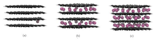
Fig. 4 Significant geometry optimised GIC structures from Li intercalation with Li placement restrictions (cf. 3.5), using PBE with the D2 correction term. Li atoms are in pink, C atoms in black, and H atoms in white. Images of all structures can be found in our ESI.† (a) 1st lithiation, Li atoms fill the central layer after this point. (b) 29th lithiation, Li atoms start filling the central layer after this point. (c) 60th lithiation is the theoretical maximum lithiation.
