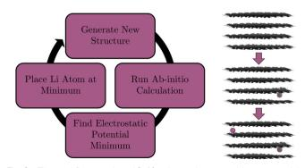
Fig. 2 The workflow employed (left) to intercalate a graphite nanoparticle (right) with Li atoms using the electrostatic potential as a guide for Li placement. Li atoms are in pink, C atoms in black, and H atoms in white.
