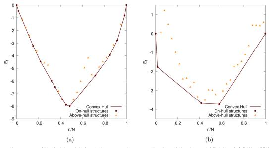
Fig. 10 The formation energy of the Li intercalated graphite nanoparticles as a function of the degree of lithiation (n/N). N=60 for our graphite nanoparticle, cf. Section 2.5 The Li intercalation proceeds via the convex hull (shown as brown line). The points on the convex hull (shown as brown circles) are the ground-states. The structures above the convex hull are shown with yellow triangles. Two different DFT functionals are considered: (a) PBE-D2 and (b) optPBE.
