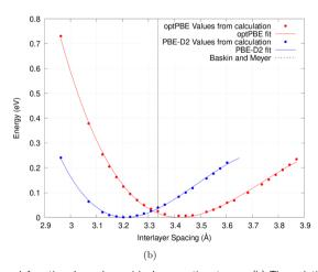
Fig. 1 (a) Periodic graphite structure used to test various non-local functionals and empirical correction terms. (b) The relationship between the interlayer spacing of bulk graphite and the total energy. A third-order Birch-Murnaghan equation of state was used to fit this plot. Results of the optPBE non-local functional and PBE with the D2 correction term are shown.<sup>63,65</sup> Experimental results by Baskin and Meyer are also shown.<sup>68</sup>
