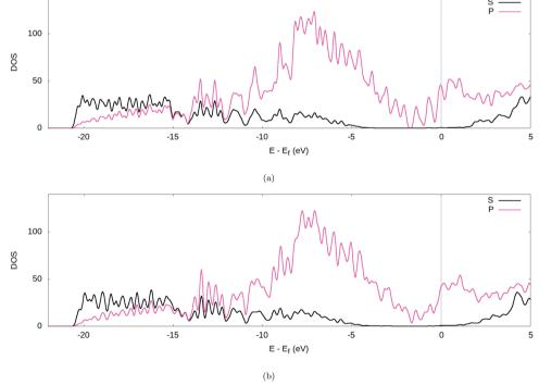
Fig. 8 PDOS of the fully lithiated graphite nanoparticle, for our (a) PBE-D2 and (b) optPBE calculations.
