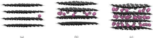
Fig. 5 Significant geometry optimised GIC structures from Li intercalation with Li placement restrictions (cf. 3.5), using the optPBE correction functional. Li atoms are in pink, C atoms in black, and H atoms in white. Images of all structures can be found in our ESI.† (a) 1st lithiation, Li atoms fill the upper and lower layers after this point. (b) 12th lithiation, Li atoms start filling the upper and lower layers after this point. (c) 60th lithiation is the theoretical maximum lithiation
