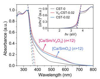
Fig. 5 UV-Vis absorption spectra of CaTiO<sub>3</sub>:Sm<sup>3+</sup>. Inset shows plots of  $(\alpha h \nu)^2 - (h \nu)$  based on the direct optical band gap.
