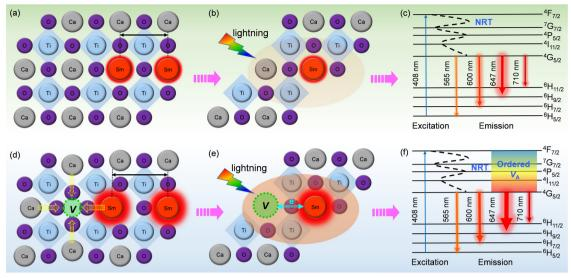
Fig. 6 Schematic diagram of PL emission mechanisms. (a-c) CST-0.02; (d-f) VA-CST-0.02. "NRT" in c and f denotes "non-radiative transition".
