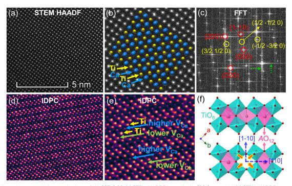
Fig. 4 Atomic-scale structural characterizations of  $V_A$ -CST-0.02. (a) STEM-HADDF image in the [001] zone axis; (b) STEM-HADDF image with atomic arrangements; (c) FFT pattern of STEM-HADDF image; (d) iDPC-STEM image in the [001] zone; (e) partial enlargement of (d); (f) the structures around dopants Sm<sup>3+</sup> and  $V_A$  in CST-x and VA-CST-x.
