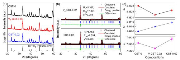
Fig. 3 Phase and structural characterizations of the undoped and A-site  $Sm^{3+}$ -doped CaTiO<sub>3</sub>. (a) Measured XRD patterns, which are presented in the form of logarithmic intensity to clearly demonstrate the tiny diffraction lines; (b) Rietveld-refined XRD patterns; (c) unit cell parameters (a, b, c) as a function of composition.
