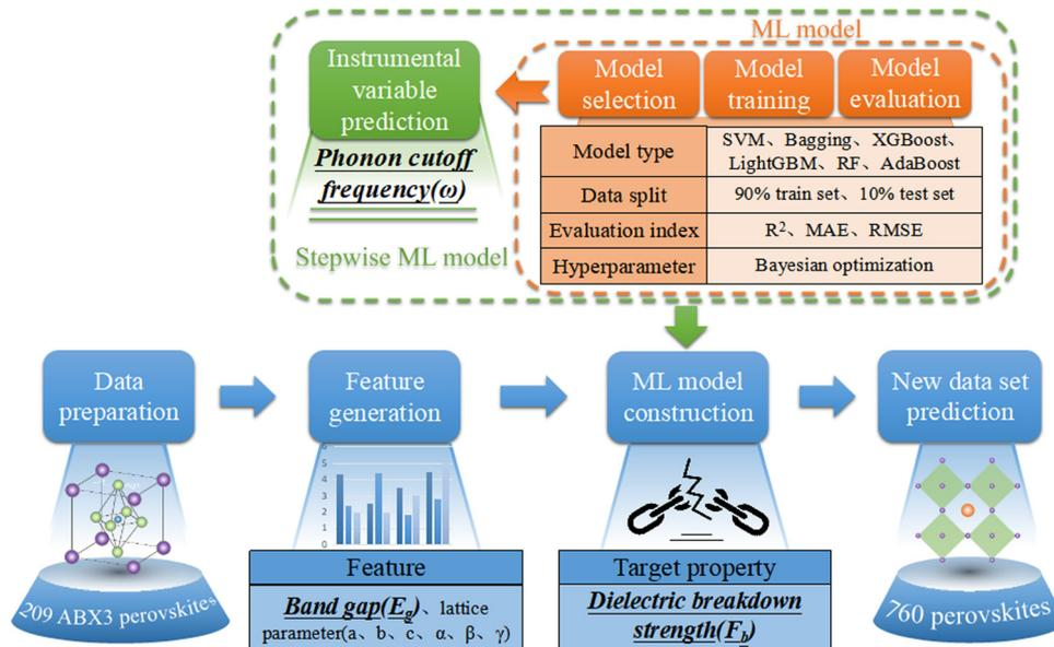
**Fig. 1** Machine learning flow chart. It can be divided into four parts: data preparation, feature generation, machine learning model construction and new data set prediction. Machine learning model construction used a stepwise method and can be divided into three parts: model selection, model training and model evaluation. The model is used to predict the phonon cutoff frequency ( $\omega$ ) and dielectric breakdown strength ( $F_b$ ) of materials.
