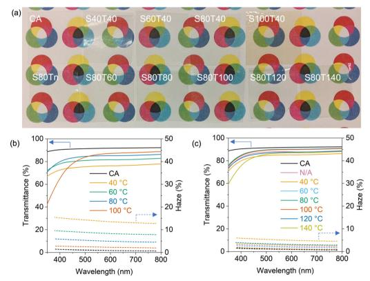
Fig. 5 Photographs (a), transmittance (solid line) and haze (dash line) spectra (b and c) for uncoated CA and coated films with different spray coating temperature (b) and different thermal treatment temperature (c). 'N/A' in c represents sample S80Tn without being thermally treated.
