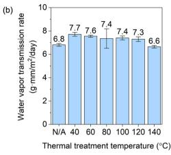
Fig. 4 Water vapor transmission rate values for coated films with different spray coating temperatures and a controlled thermal treatment temperature (40 °C) (a) and varying thermal treatment temperatures and a controlled spray coating temperature (80 °C) (b). 'N/A' represents sample S80Tn without being thermally treated.
