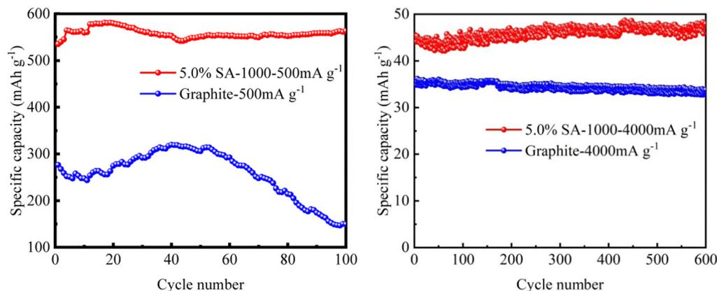
Fig. 9 The cyclic properties of the 5.0% SA-1000 composite and graphite samples (a) 500 mA g<sup>-1</sup> and (b) 4000 mA g<sup>-1</sup>.
