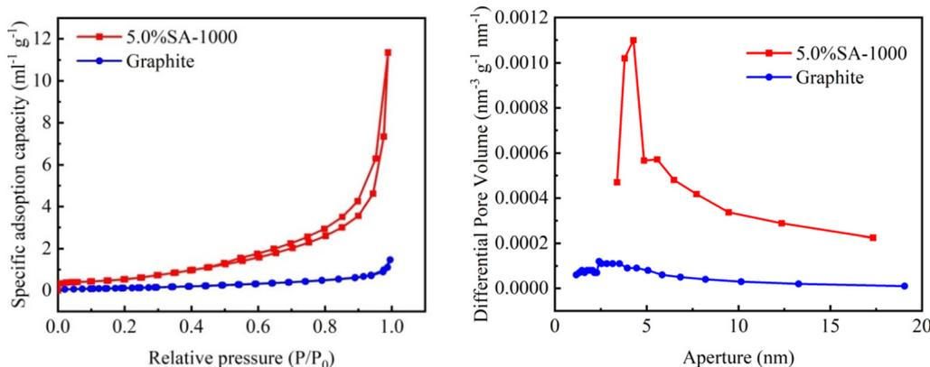
Fig. 4 BET for the best coating of the 5.0% SA-1000 and graphite samples.
