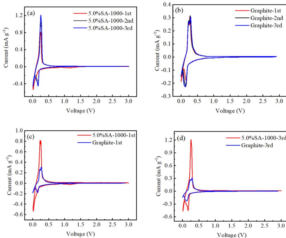
Fig. 10 Cyclic voltammogram of (a) the composite material 5.0% SA-1000 (b) graphite sample. (c) A comparison of the first ring of the 5.0% SA-1000 and graphite samples. (d) A comparison of the tail ring of the 5.0% SA-1000 and graphite samples.
