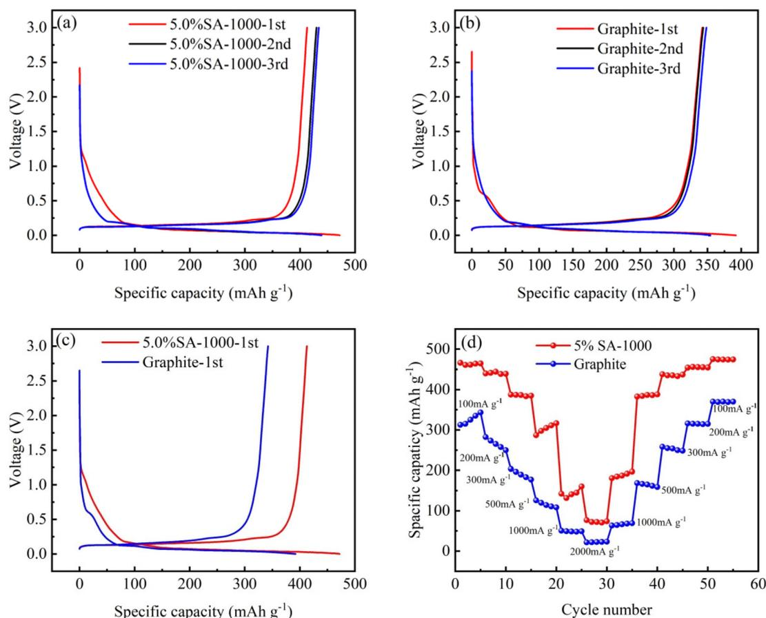
**Fig. 8** Charge–discharge curve for (a) 5.0% SA-1000 and (b) graphite samples. (c) First-ring charge–discharge comparison curve. (d) Rate performance curve of the composite sample 5.0% SA-1000 and graphite sample.
