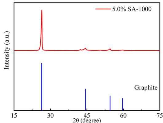
Fig. 5 XRD of the 5.0% SA-1000 composite and graphite sample.
