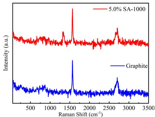
Fig. 6 RAMAN of the 5.0% SA-1000 composite and graphite sample.
