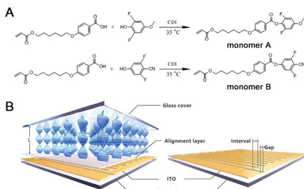
**Fig. 1** Synthetic routes of monomer A and monomer B (A); structure diagram of horizontally aligned CLCP coating over the transparent interdigitated comb-shape electrode (conducting layer: indium tin oxide (ITO); gap: 30  $\mu\text{m}$ ; interval: 30, 60 and 120  $\mu\text{m}$ ) (B).
