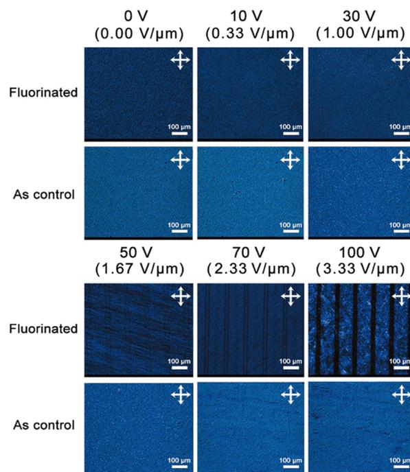
Fig. 2 POM images of horizontally aligned fluorinated CLCP coating with a thickness of 5  $\mu\text{m}$  at 50 °C under an applied DC field of different voltages (3 cm × 3 cm ITO electrode substrate: gap, 30  $\mu\text{m}$ ; interval, 60  $\mu\text{m}$ ). Similar fluorine-free CLCP used as a control.
