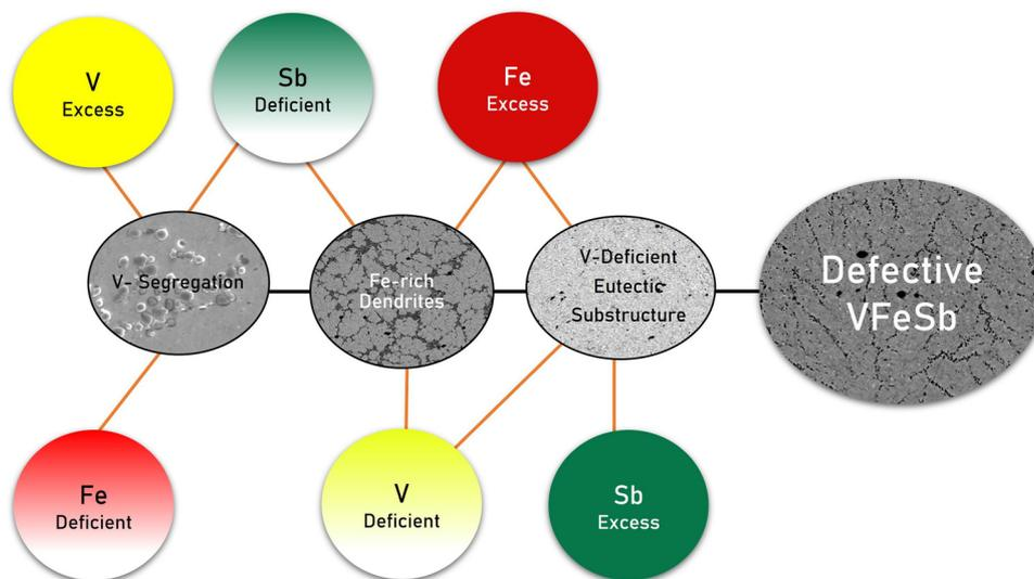
Fig. 7 Schematic fishbone diagram showing the predominant granular defects, *i.e.* V-segregates, V-deficient eutectic substructure, and Fe-rich dendrites observed in VFeSb half-Heusler alloys, and the stoichiometric origin behind their formations.
