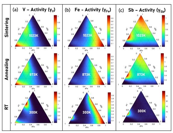
The activity coefficients of (a) V, (b) Fe, and (c) Sb at room temperature (300 K), annealing (873 K), and sintering (1023 K) temperature in VFeSb Fig. 9 alloys.
