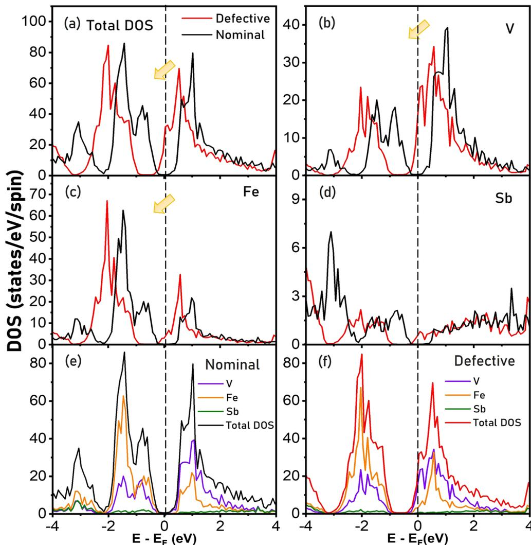
Fig. 4 Comparison of (a) total and site-decomposed, (b) V-site, (c) Fe-site, and (d) Sb-site density of states of nominal and defective compositions. The total and atom-projected density of states for (e) nominal and (f) defective VFeSb compositions.
