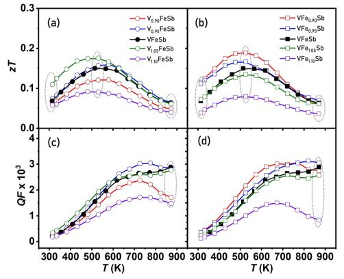
Fig. 10 Temperature-dependent thermoelectric (a and b) figure-of-merit (zT) and (c and d) quality factor of  $V_{1+x}$ Fe<sub>1+y</sub>Sb (-0.1 < x, y < 0.1) half-Heusler alloys.
