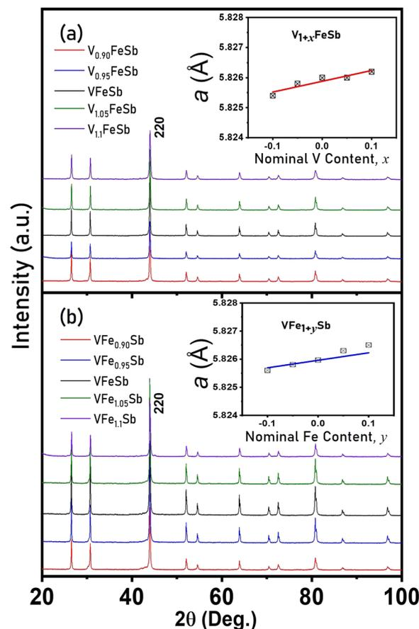
Fig. 1 X-Ray diffraction patterns of (a)  $V_{1+x}FeSb$  and (b)  $VFe_{1+y}Sb$  half-Heusler alloys along with a lattice constant with varying V and Fe stoichiometry ( $-0.1 < x, y < 0.1$ ) are shown in the inset.
