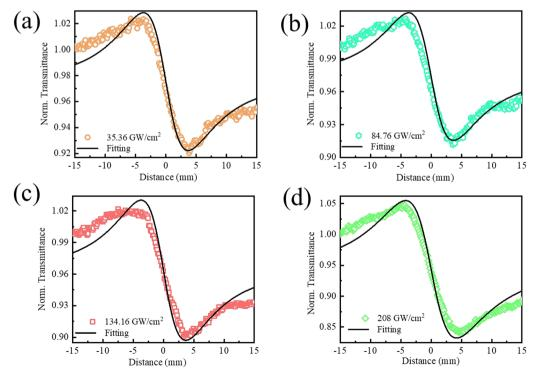
Fig. 6 Closed aperture (CA) Z-scan curves captured at an excitation wavelength of 800 nm for (a) 35.36, (b) 84.76, (c) 134.16 and (d) 208 GW cm<sup>-2</sup> input intensities.
