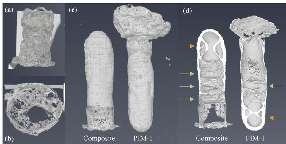
Fig. 5 XRCT renderings of (a) composite foam exterior and (b) cross section. Both PIM-1 and composite monolith (c) exteriors and (d) cross sections. Arrows indicate repeated hour glass (yellow) and planar (green) void geometries believed to arise from convection in a hemisphere during freezing.
