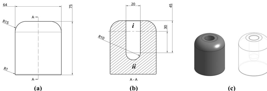
Fig. 3 (a and b) Projection drawings of mould (dimensions in mm) and (c) renderings from *Onshape*. Dimensions are in mm with 'R' denoting 'radius'. To ease discussion, i and ii indicate regions of excess cavity and mould mass, respectively.
