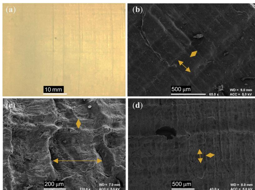
**Fig. 6** (a) Layers of cured resin on the mould exterior arise from the resolution of the SLA printer laser and are (b) visible under SEM. Orange arrows indicate repeating  $0.3$  by  $0.1 \text{ mm}$  checker patterns. This has then been transferred to the exterior of (c) composite and (d) PIM-1 monoliths during casting.
