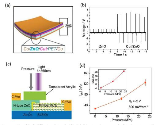
Fig. 26 (a) Schematic presentation of the ZnO/Cul-based piezoelectric photodetector and nanogenerator (b) output voltage of the pristine and ZnO-Cul-based devices. Reprinted with permission from ref. 285. Copyright 2016 Elsevier. (c) Piezotronics device based on ZnO and MoS<sub>2</sub>. (d) Piezophotoresponse from the piezotronics FET device. Reprinted with permission from ref. 288. Copyright 2016 John Wiley and Sons.
