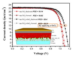
Fig. 10 Cross-sectional SEM image of the perovskite solar cell based on mp-TiO<sub>2</sub>/a-SnO<sub>2</sub>. J-V curves for mp-TiO<sub>2</sub> and mp-TiO<sub>2</sub>/a-SnO<sub>2</sub> along with the power conversion efficiencies. Inset shows a schematic of a perovskite solar cell based on mp-TiO<sub>2</sub>/a-SnO<sub>2</sub>. Reprinted with permission from ref. 227. Copyright 2018 American Chemical Society.
