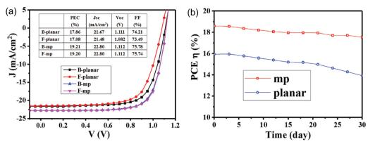
Fig. 11 (a) J-V graphs obtained of the planar SnO<sub>2</sub> and mp SnO<sub>2</sub> PSCs from under backward and forward voltage scanning. (b) PCEs of the planar SnO<sub>2</sub> and mp SnO<sub>2</sub> PSCs monitored every 3 d; the measurement was performed under AM 1.5G with input solar power  $P_{in}$  of 100 mW cm<sup>-2</sup>. Reprinted with permission from ref. 224. Copyright 2018 John Wiley and Sons.
