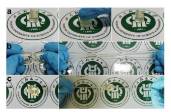
Fig. 3 The poly(AM-co-AA)/GQD hydrogels (1 wt% GQDs) exhibited significant mechanical toughness ((a) compressed and released, (b) crossbent and stretched, and (c) knotted and stretched).
