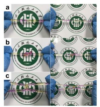
Fig. 5 Images showing the poly(AM-co-AA)/GQD nanocomposite gels (1 wt% GQDs) after being cut and then healed for 10 h. The healed sample could be (a) stretched, (b) knotted and stretched, and (c) cross-bent and stretched without breaking
