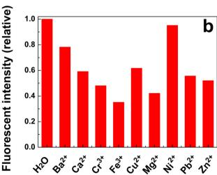
Fig. 9 Fluorescence response of the poly(AM-co-AA)/GQD nanocomposite hydrogels (1 wt% GQDs) to different ions dissolved in deionized water: (a) fluorescence spectra and (b) corresponding relative fluorescence
