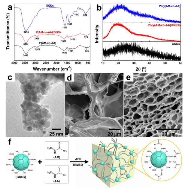
Fig. 2 (a) FTIR spectrum, (b) XRD patterns, and (c) TEM image of poly(AM-co-AA)/GQD nanocomposite hydrogels (1 wt% GQDs); (d and e) SEM photographs of poly(AM-co-AA) and poly(AM-co-AA)/GQD hydrogels (1 wt% GQDs), respectively; (f) schematic representation of the formation of poly(AM-co-AA)/GQD nanocomposite hydrogels and the supposed interactions between the polymer chains and the GQDs (enlarged drawing).
