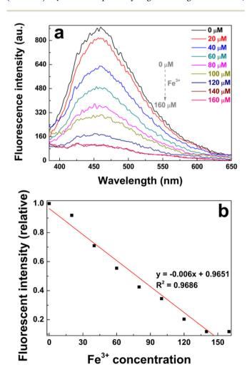
Fig. 7 (a) Fluorescence spectra and (b) the relationship between the fluorescence intensity of poly(AM-co-AA)/GQD nanocomposite hydrogels (1 wt% GQDs) and the concentration of Fe<sup>3+</sup>.
