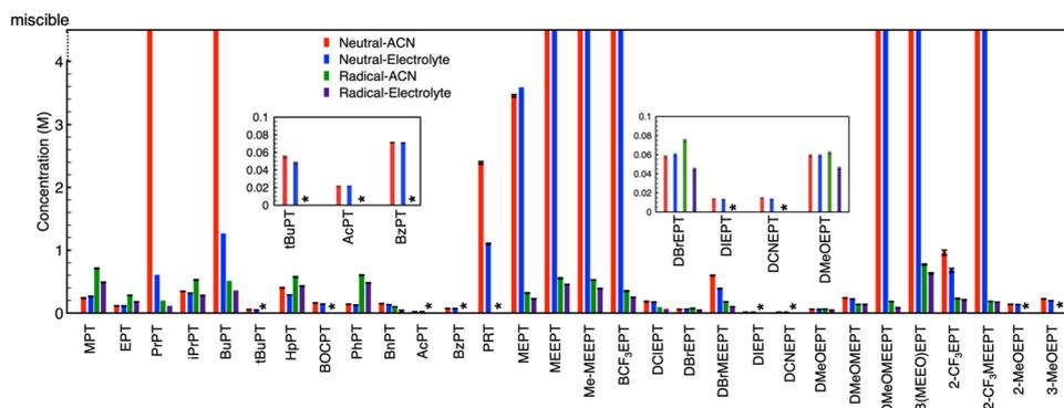
Fig. 4 Solubility of various phenothiazines in their neutral and charged forms in acetonitrile and 0.5 M TEABF<sub>4</sub>/ACN labeled “electrolyte” (\*: unstable radical cations failed to be isolated as solids).
