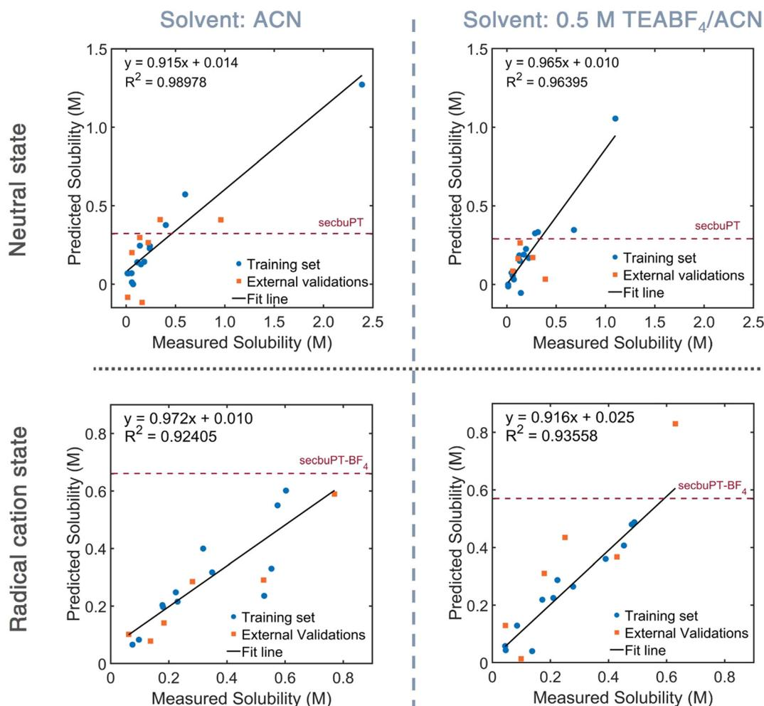
Fig. 5 Predictive models for neutral and charged of *sec*-butylPT in ACN and 0.5 M TEABF<sub>4</sub> in ACN.
