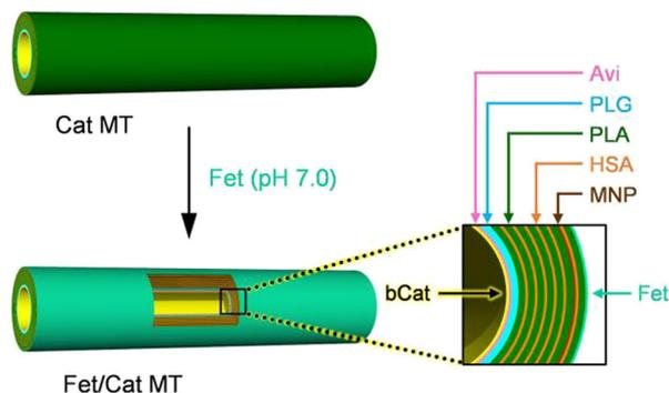
Fig. 1 Preparation and stratiform structure of the protein MT motor with a Cat engine layer as an internal wall and Fet exterior surface: Fet/PLA/HSA/MNP(PLA/HSA)<sub>5</sub>PLA/PLG/Avi/bCat MT (Fet/Cat MT).
