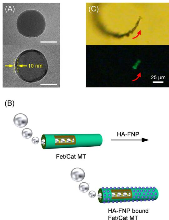
**Fig. 4** (A) TEM images of (top) unmodified FNPs and (bottom) HA-FNPs (bar: 50 nm). (B) Schematic illustration of HA-FNPs capturing a bubble-propelled Fet/Cat MT. (C) Snapshots taken from Video S3 (ESI<sup>†</sup>) of microscopic observations of self-propelled HA-FNP bound Fet/Cat MT by ejecting O<sub>2</sub> bubbles in PB solution (pH 7.0, 2 wt% H<sub>2</sub>O<sub>2</sub>, and 0.1 wt% Triton X-100) at 25 °C under (top) bright field mode and (bottom) fluorescence mode.
