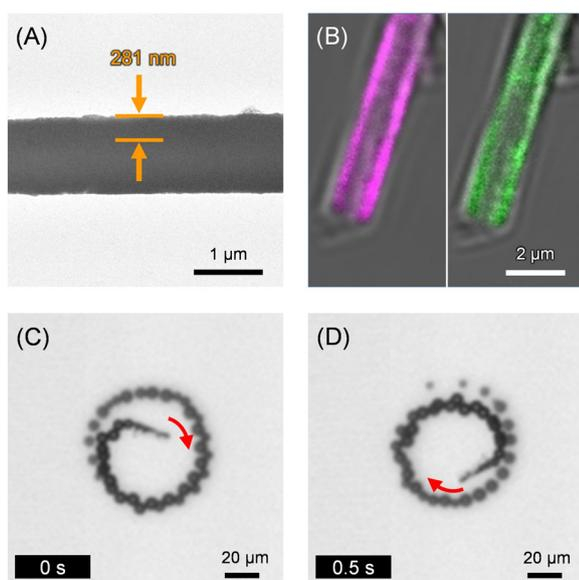
Fig. 2 (A) The TEM image of Fet/Cat MT. (B) The CLSM images of CyFet/FCat MT (left –  $\lambda_{\text{ex}}$ , 633 nm for CyFet; right –  $\lambda_{\text{ex}}$ , 488 nm for FCat). (C and D) Snapshots taken from Video S1 (ESI<sup>†</sup>) of microscopic observations of self-propelled Fet/Cat MT by ejecting O<sub>2</sub> bubbles in PB solution (pH 7.0, 2 wt% H<sub>2</sub>O<sub>2</sub>, and 0.1 wt% Triton X-100) at 25 °C under bright field mode.
