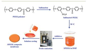
Fig. 5 Schematic preparation of SPEEK membranes.
