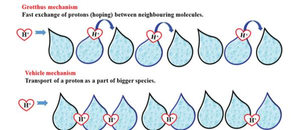
Fig. 6 Proton transport mechanism in the fuel cell
