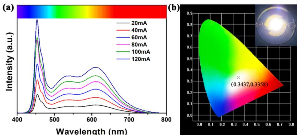
Fig. 7 (a) Emission spectra of the G-CD-based WLEDs at different currents; and (b) CIE chromaticity diagram of the G-CD-based WLEDs at 100 mA current.
