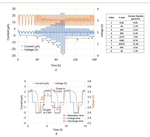
Fig. 6 Current and voltage profiles for Al/C|[LFP(98.5%)/C(1.5%)] +  $xLi_3OCl|Li$  electrochemical cell at 100 °C: (a) charge and discharge cycles at 0.6C with a fixed 1 h relaxation time, and (b) representation of a test schedule for current and voltage as a function of time at various C-rates.
