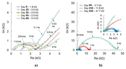
Fig. 8 AC impedance data of a cell Al/C|[LFP(98.5%)/C(1.5%)] +  $xLi_3OCl|Li_3OCl|Li$  tested at 100 °C. The scatter with markers plot corresponds to experimental values, while solid lines represent fitted data. (a) Data (0–60 days) where no significant change in charge-transfer resistances was detected, and (b) Nyquist plots of the last three measurements showed a significant increase in the cell resistance.
