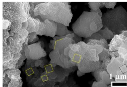
Fig. 4 Representative FESEM image of SnO<sub>2</sub> fab-fracs showing square-shaped building blocks. Reprinted by permission from Springer Nature Customer Service Centre GmbH: Springer, Journal of Sol–Gel Science and Technology, Large-scale growth of tin oxide fabricated fractals, Vishal Kamathe and Rupali Nagar, Copyright (2022) Springer Nature Switzerland AG, Part of Springer Nature.<sup>20</sup>
