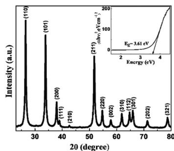
Fig. 3 X-Ray diffractogram of SnO<sub>2</sub> fab-fracs showing peaks corresponding to different Miller indices. The inset shows the bandgap of 3.61 eV as estimated from Tauc plot. Reprinted by permission from Springer Nature Customer Service Centre GmbH: Springer, Journal of Sol–Gel Science and Technology, Large-scale growth of tin oxide fabricated fractals, Vishal Kamathe and Rupali Nagar, Copyright (2022) Springer Nature Switzerland AG, Part of Springer Nature.<sup>20</sup>
