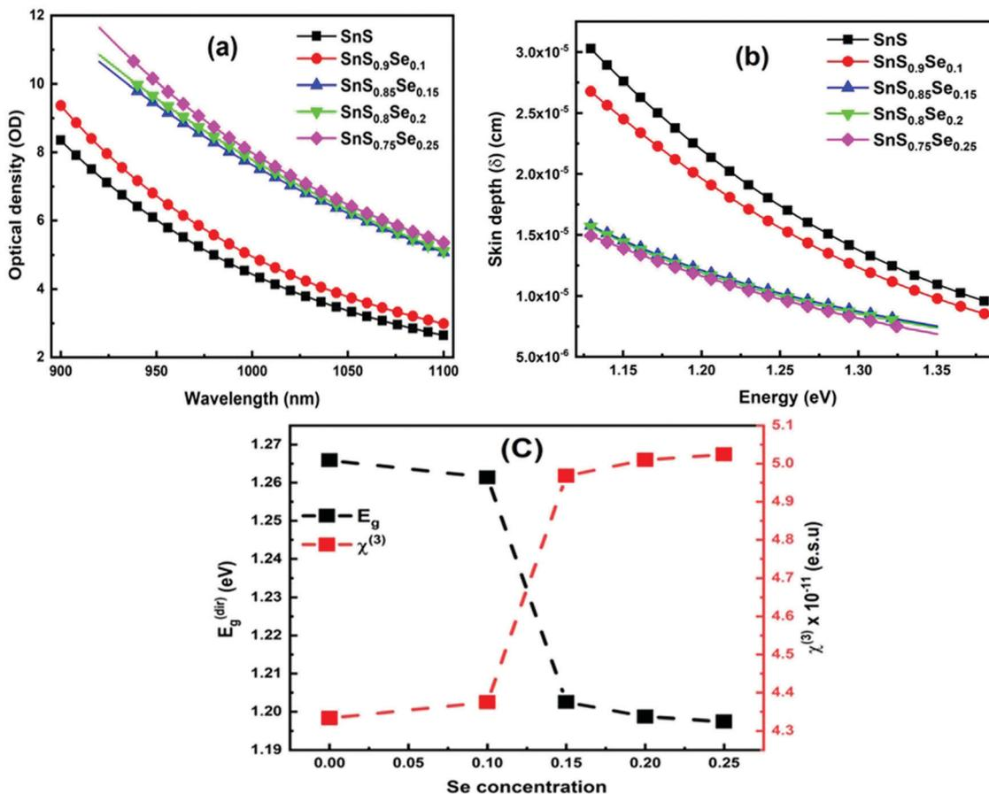
Fig. 4 (a) Change in the optical density of SnS<sub>1-x</sub>Se<sub>x</sub> (x = 0, 0.1, 0.15, 0.2, 0.25) thin films, (b) skin depth of SnS<sub>1-x</sub>Se<sub>x</sub> with energy, and (c) variation of  $E_g$  and  $\chi^{(3)}$  with Se doping concentration.
