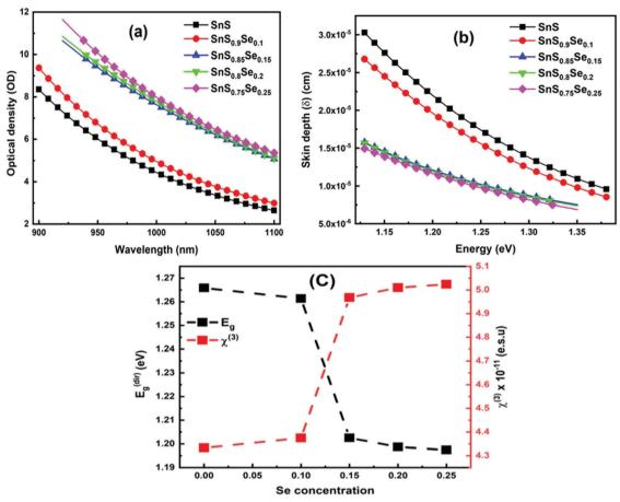
Fig. 4 (a) Change in the optical density of  $SnS_{1-x}Se_x$  (x = 0, 0.1, 0.15, 0.2, 0.25) thin films, (b) skin depth of  $SnS_{1-x}Se_x$  with energy, and (c) variation of  $E_q$ and  $\chi^3$  with Se doping concentration
