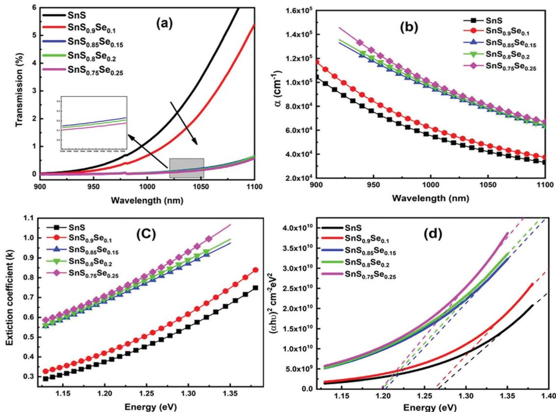
Fig. 3 (a) Transmittance spectra of  $\text{SnS}_{1-x}\text{Se}_x$  ( $x = 0, 0.1, 0.15, 0.2, 0.25$ ) thin films, (b) change in the absorption coefficient ( $\alpha$ ) with Se concentration, (c) variation of the extinction coefficient ( $k$ ), and (d) estimation of the direct bandgap for different Se concentration films.
