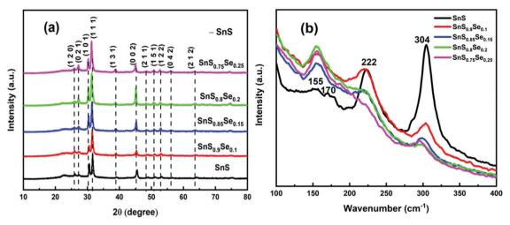
Fig. 1 (a) XRD pattern presenting different phases and (b) Raman spectra of  $SnS_{1-x}Se_x$  (x = 0, 0.1, 0.15, 0.2, 0.25) thin films
