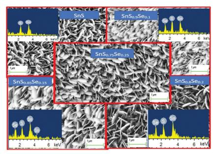
Fig. 2 FESEM images of  $SnS_{1-x}Se_x$  (x = 0, 0.1, 0.15, 0.2, 0.25) thin films and their corresponding EDX images (inset)
