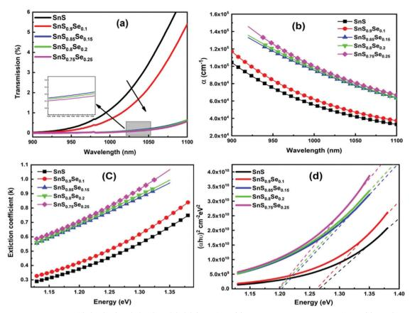
Fig. 3 (a) Transmittance spectra of  $SnS_{1-x}Se_x$  (x = 0, 0.1, 0.15, 0.2, 0.25) thin films, (b) change in the absorption coefficient ( $\alpha$ ) with Se concentration, (c) variation of the extinction coefficient (k), and (d) estimation of the direct bandgap for different Se concentration films.
