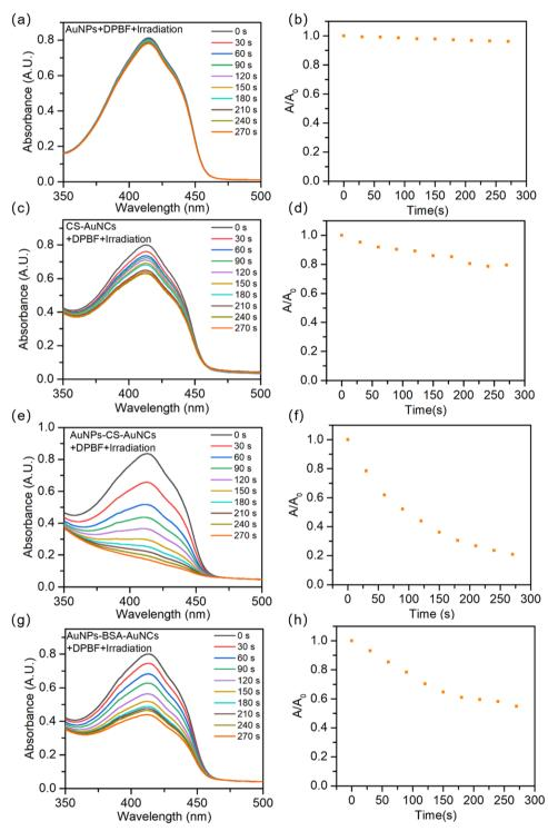
Fig. 4 Absorption spectra of DPBF under 570 nm irradiation at different times and absorbance ratio of the irradiation time maximum absorbance (At) to the time zero maximum absorbance (A0) for (a), (b) AuNPs, (c), (d) CS-AuNCs, (e), (f) AuNPs-CS-AuNCs and (g), (h) AuNPs-BSA-AuNCs.
