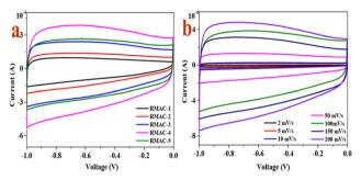
Fig. 4 (a) CV curves of RMAC samples prepared under different ratios of precursor/KOH at 100 mV s $^{-1}$  and (b) CV curves of RMAC-4 at different scan rates.
