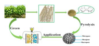
Fig. 7 Schematic illustration of the formation of the supercapacitor.
