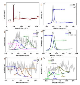
Fig. 3 (a) XPS survey spectrum of RMAC-4, (b) high resolution C1s of RMAC-4;,(c) high resolution N1s of RMAC-4, (d) high resolution O1s of RMAC-4, (e) high resolution P2p of RMAC-4, and (f) high resolution S2p of RMAC-4
