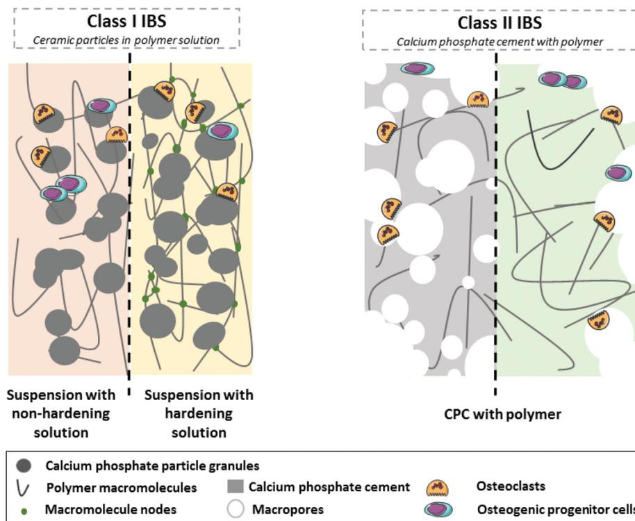
**Fig. 1** The two classes of IBS present different osteoconduction mechanisms: for Class I, calcium phosphate supports are made of divided ceramics (thermally-sintered particles, resulting in high density materials); for Class II, calcium phosphate supports are made of bulk cements (soft chemistry route to interlinked particles, resulting in low-density materials showing macropores).
