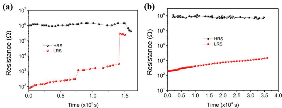
Fig. 8 Resistance state retention of (a) MemPVCell-1 and (b) MemPVCell-2. The following pulse settings were used: amplitude  $\pm 1$  V and pulse duration 500 ms. For resistance reading, a pulse with the amplitude of  $\pm 20$  mV and the duration of 10 ms every 5 s was used.
