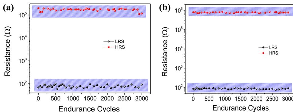
Fig. 7 Cycling endurance of (a) MemPVCell-1 and (b) MemPVCell-2. The following pulse settings were used: number of pulses up to  $3 \times 10^3$ , amplitude  $\pm 1$  V, pulse duration 100 ms. For resistance reading, a pulse with the amplitude of  $\pm 10$  mV and the duration of 10 ms was used.
