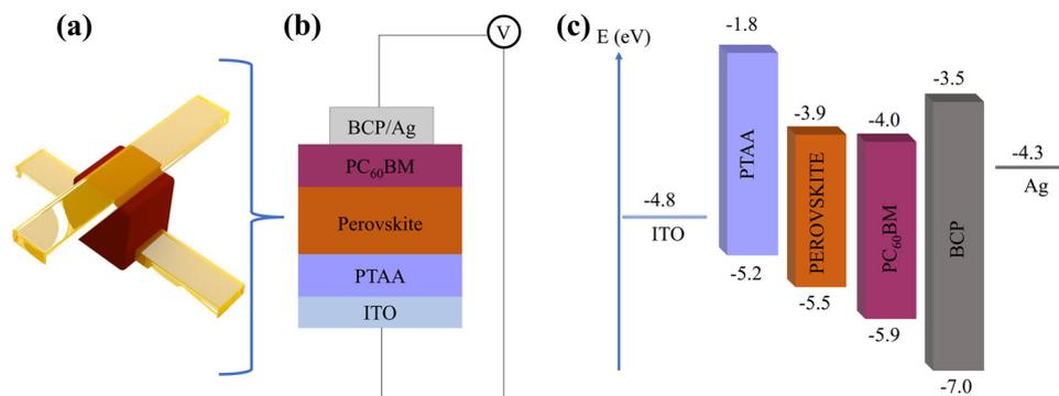
**Fig. 1** MemPVCell schematic structure and energy bands. (a) Schematic illustration of the MemPVCell device having an inverted PSC structure and (b) consisting of a glass/ITO/PTAA/Perovskite/ $\text{PC}_{60}\text{BM}$ /BCP/Ag material stack. (c) Graphic representation of the layer's energy diagram.
