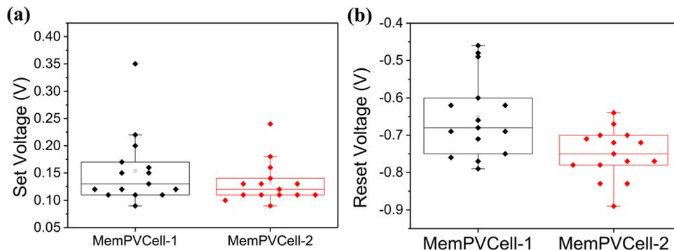
Fig. 5 Resistive switching voltage statistics for 15 MemPVCell-1 (black data) and 15 MemPVCell-2 devices (red data). MemPVCell-1 devices exhibit a slightly higher  $V_{\text{set}}$  while having a slightly lower  $V_{\text{reset}}$  compared to MemPVCell-2.  $I_{\text{cc}} = 10$  mA and a scanning rate of  $10$  mV  $\text{s}^{-1}$  were used.
