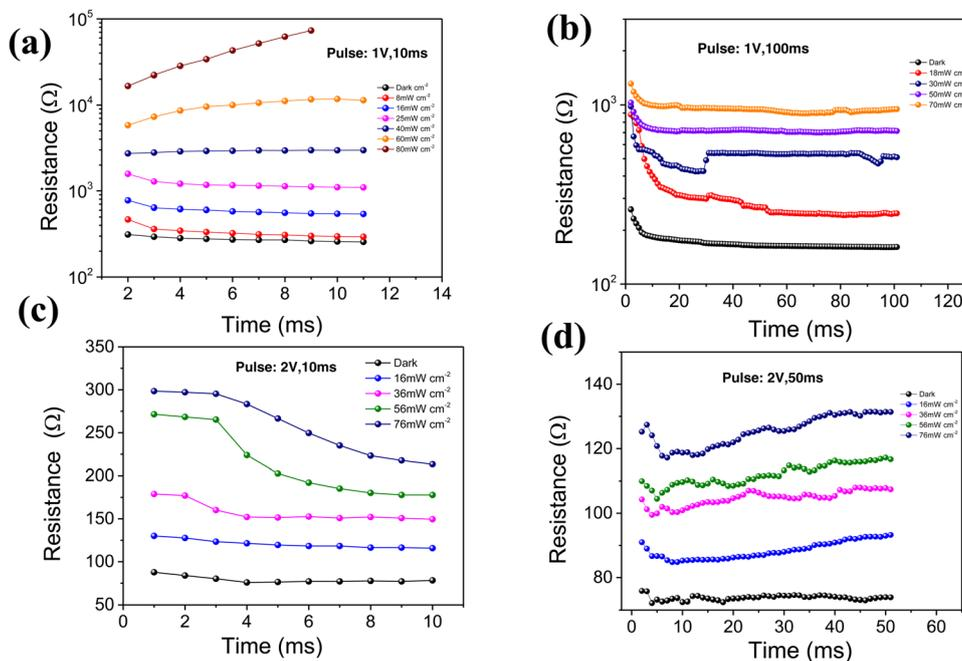
Fig. 6 Light tuning of the resistance state of MemPVCell-1 under different illumination and electric pulse conditions. An electric pulse of the amplitude and duration of (a) 1 V, 10 ms, (b) 1 V, 100 ms, (c) 2 V, 10 ms, and (d) 2 V, 50 ms was applied to set the sample close to the LRS. Light illumination was varied from dark conditions up to  $80$   $\text{mW cm}^{-2}$ .
