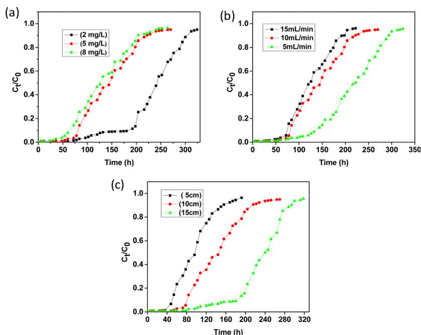
Fig. 9 Breakthrough curves for the adsorption of fluoride (a) at different initial concentrations, (b) at different flow rates and (c) at different bed heights.
