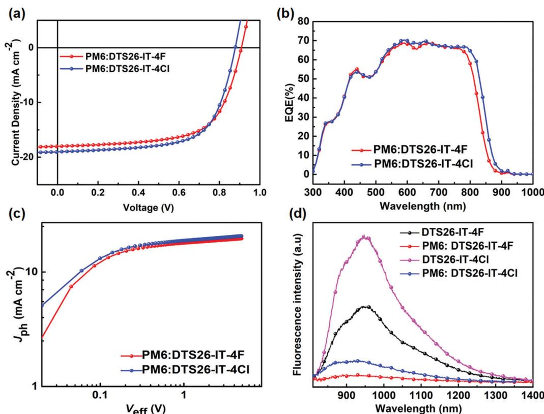
Fig. 2 (a)  $J$ – $V$  curves, (b) EQE curves, and (c)  $J_{ph}$ – $V_{eff}$  curves of the optimal PM6:DTS26-IT-4F and PM6:DTS26-IT-4Cl based OSCs. (d) PL spectra of the optimal PM6:DTS26-IT-4F and PM6:DTS26-IT-4Cl blend films, and DTS26-IT-4F and DTS26-IT-4Cl neat films excited at 780 nm.
