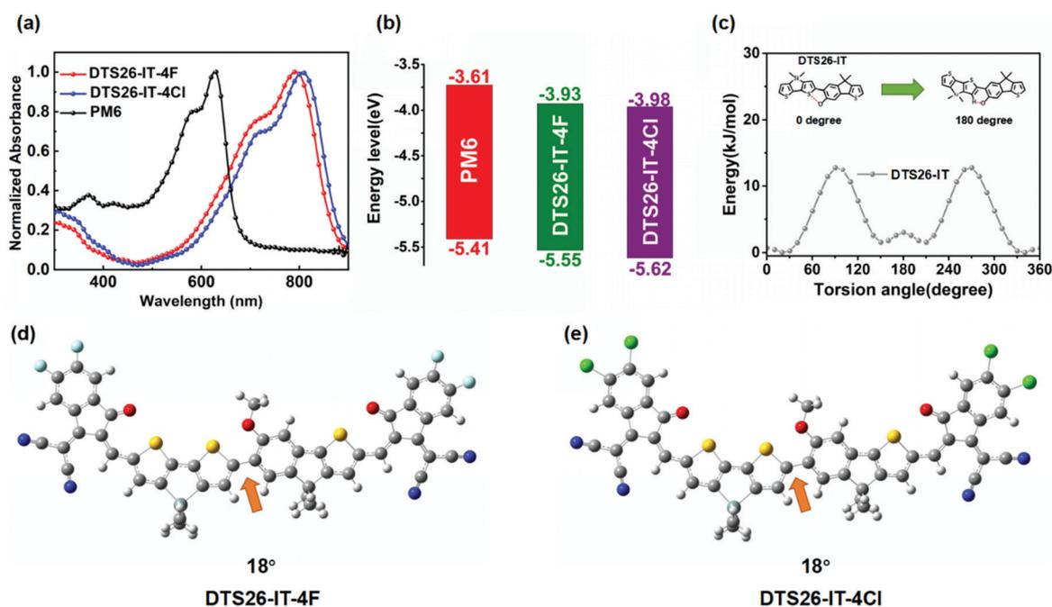
Fig. 1 (a) Normalized UV-Vis-NIR absorption spectra, (b) energy level diagrams of PM6, **DTS26-IT-4F** and **DTS26-IT-4Cl**, and (c) potential energy surface scan of the rotamer **DTS26-IT**, (d) molecular geometry of **DTS26-IT-4F** and (e) molecular geometry of **DTS26-IT-4Cl** calculated by DFT.
