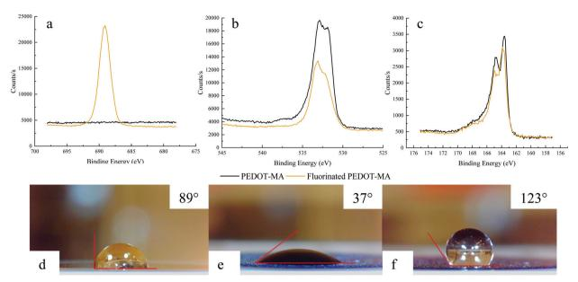
Fig. 9 (Top) XPS spectra of (a) fluorine, (b) oxygen, and (c) sulfur for PEDOT-MA films before and after fluorination and (bottom) Contact angle measurements of (d) pristine crystal, (e) PEDOT-MA before post-process, and (f) PEDOT-MA after post-process. Corresponding contact angles are marked in pictures.
