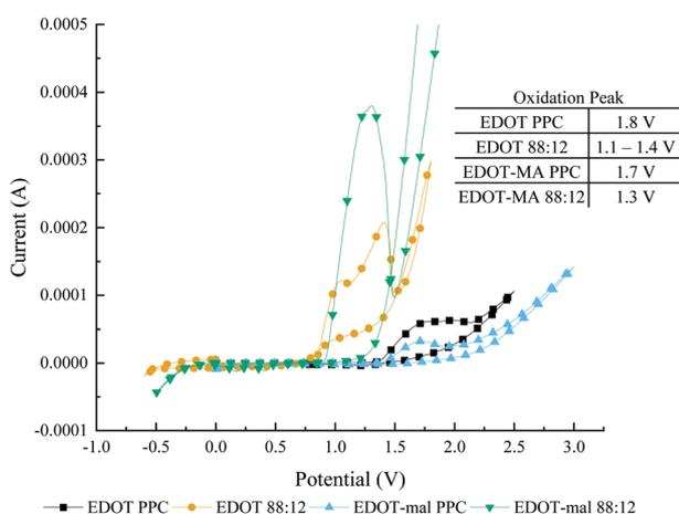
Fig. 1 Cyclic voltammety polymerization by variation in solvent from propylene carbonate to 88 : 12,  $\text{H}_2\text{O}:\text{PPC}$  mixed solvent. Peaks determined by local maximums.
