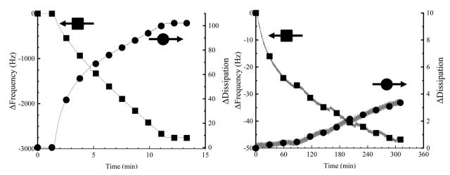
Fig. 8 Change in frequency ( $\Delta f$ ) and change in dissipation ( $\Delta D$ ) for (left) PEDOT-MA deposition and (right) fluorothiol functionalization.
