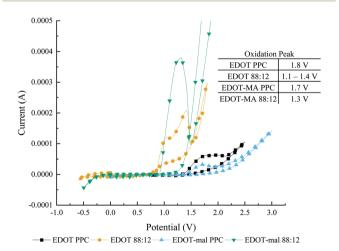
Fig. 1 Cyclic voltammetry polymerization by variation in solvent from propylene carbonate to 88:12, H<sub>2</sub>O:PPC mixed solvent. Peaks determined by local maximums
