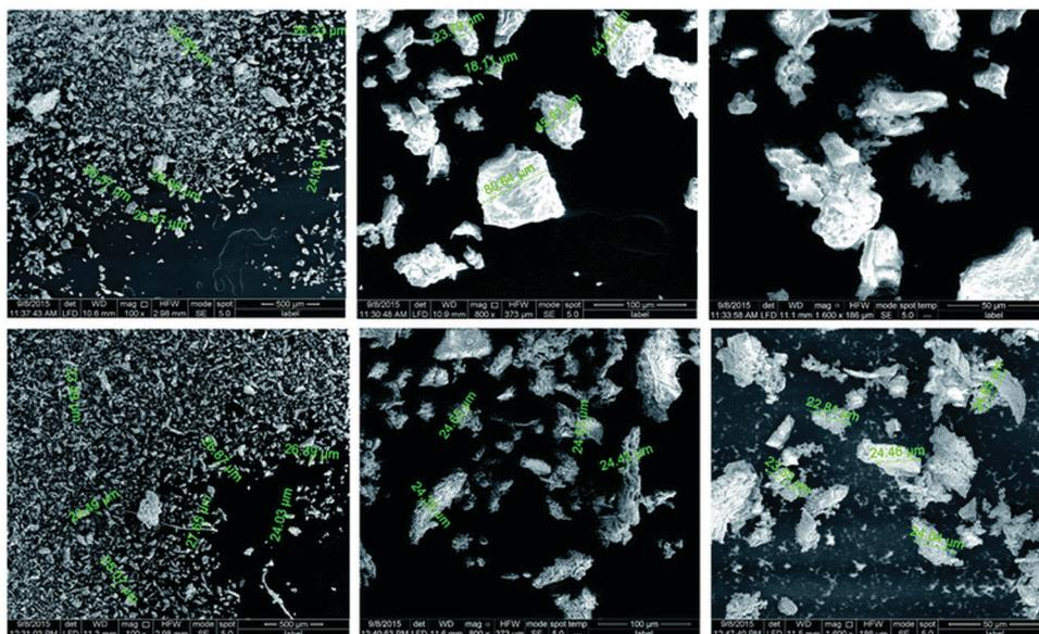
Fig. 8 SEM images of unloaded MCS-GMA-I (top), and loaded MCS-GMA-I (bottom).<sup>67</sup>
