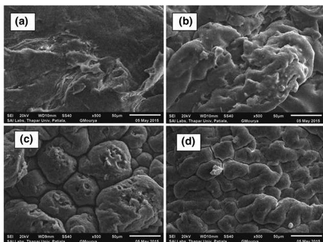
Fig. 18 SEM of (a) pristine TS, (b) grafted-TS (% grafting, 51.8%), (c) sulphonic acid grafted-TS (% conversion, 15.9%), and (d) aminated grafted-TS (% conversion, 16.2%).<sup>137</sup> Reproduced from ref. 137, with permission from Springer Nature, 2016.
