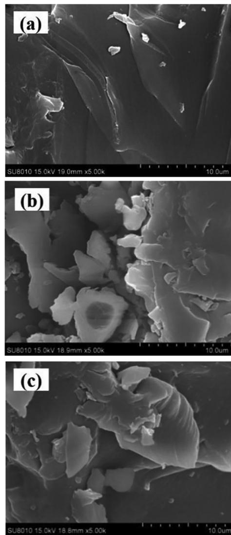
Fig. 5 Morphology of (a) CS, (b) PAA-PAM-CS, and (c) g-CS.<sup>54</sup> Reproduced from ref. 54, with permission from Elsevier, 2020.
