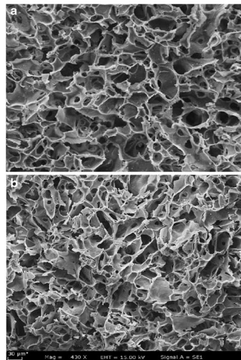
Fig. 20 SEM micrographs of the macroporous structure for (a) p(HEMA-GMA) and (b) p(HEMA-GMA)- $\text{PO}_4^{2-}$ .<sup>140</sup> Reproduced from ref. 140, with permission from Springer Nature, 2020.
