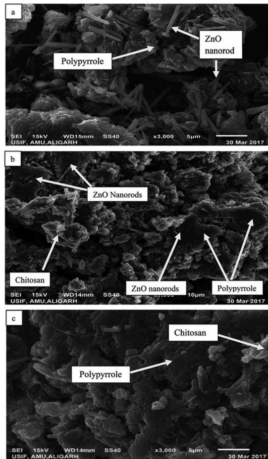
Fig. 3 SEM images of the as-prepared nanoparticles and nanocomposites: (a) Pp-Z, (b) Pp-CS-Z, and (c) Pp-CS.<sup>52</sup>
