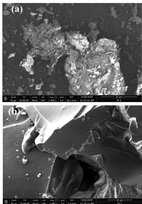
Fig. 6 Typical SEM images of polymer composite hydrogel (a) before dye adsorption, and (b) after dye adsorption.<sup>62</sup> Reproduced from ref. 62, with permission from Springer Nature, 2022.
