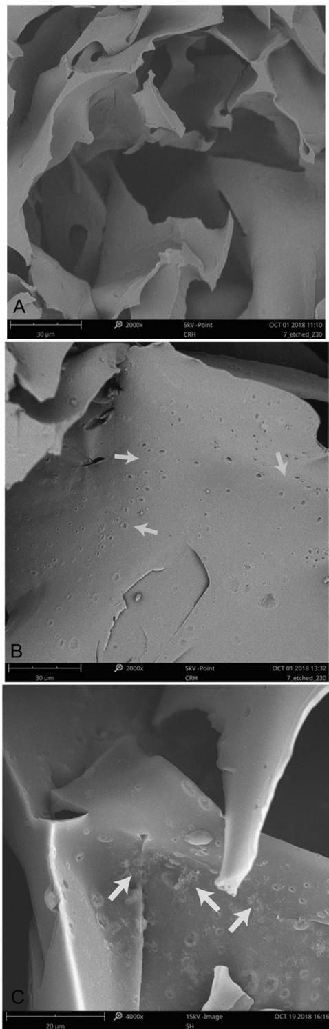
Fig. 14 SEM images of (A) unmodified poly(HEMA-GMA), (B) Cell-modified poly(HEMA-GMA), and (C) Fe(II)-immobilized poly(HEMA-GMA)-Cell cryogels.<sup>128</sup> Reproduced from ref. 128, with permission from Springer Nature, 2022.
