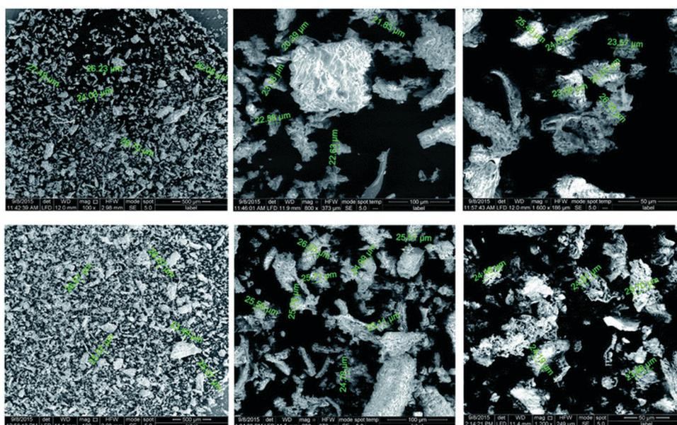
Fig. 9 SEM images of unloaded MCS-GMA-II (top), and loaded MCS-GMA-II (bottom).<sup>67</sup>
