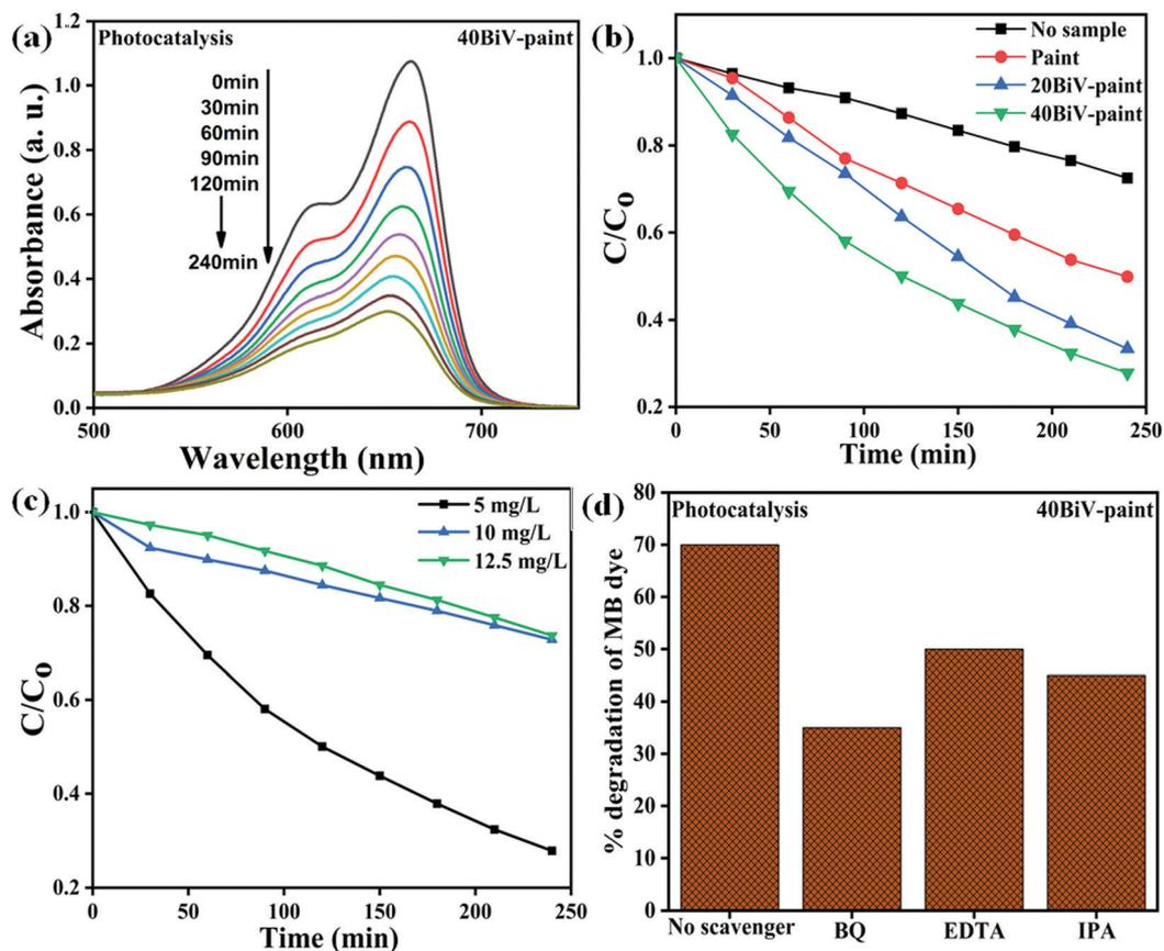
Fig. 6 (a) Absorption spectra acquired from the photocatalysis using the 40BiV-paint sample, (b)  $C/C_0$  vs. time plots acquired from photocatalysis with and without any sample use, (c)  $C/C_0$  vs. time plots acquired from photocatalysis using the 40BiV-paint sample at different MB dye concentrations (5, 10, and 12.5 mg L<sup>-1</sup>), and (d) effect of different scavengers on MB dye degradation efficiency acquired from the photocatalysis experiment using the 40BiV-paint sample.
