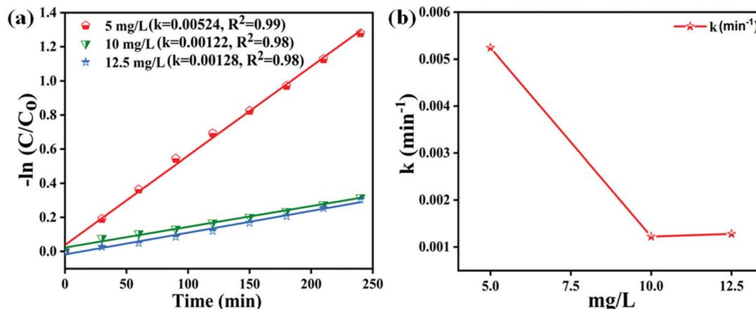
Fig. 7 (a)  $-\ln(C/C_0)$  vs. time plots for various MB dye concentrations (mg L<sup>-1</sup>) and (b) plots of kinetic rate constant ' $k$ ' vs. varied dye concentrations during photocatalysis.
