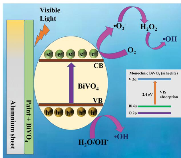
Fig. 9 Schematic mechanism for photocatalytic MB dye degradation using the BiV-paint sample.
