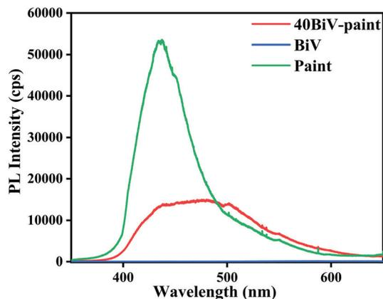
Fig. 4 Photoluminescence spectra of 40BiV-paint, BiV, and paint.
