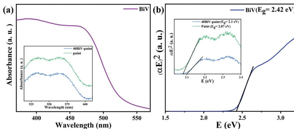
Fig. 3 (a) UV-vis absorption spectrum of BiV powder (inset graph shows the absorption edge of 40BiV-paint and paint) and (b) bandgap of BiV using Tauc plots (inset graph shows the bandgap of 40BiV-paint and paint).
